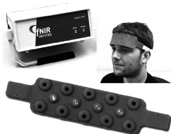
Figure 3. fNIR devices (data acquisition control box and fNIR sensor pad)
