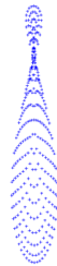
Figure 4. The ideal spot diagram for the SCOTS GMT test, an area of approximately 220×40 mm on the monitor screen.
