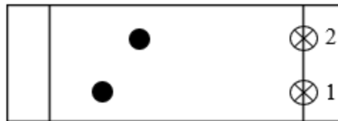
Figure 1: TLC of (1) and (2) using a 3:1 DCM/n-heptane blend-top to the left.
