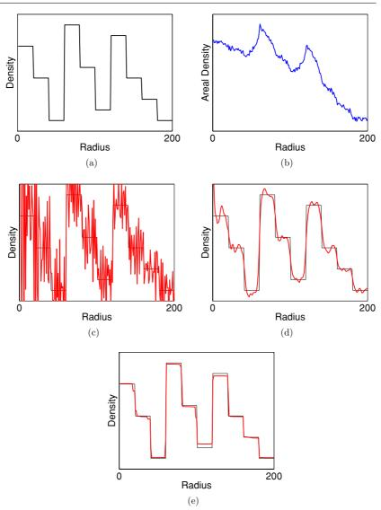
**Figure 2.** (a) Density profile; (b) Abel transform, with noise added; (c) unregularized Abel inversion; (d)  $H^1$ -regularized Abel inversion; (e) TV-regularized Abel inversion.
