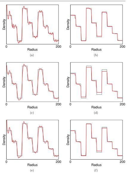
**Figure 3.** (a) Underregularized  $H^1$  Abel inversion; (b) underregularized TV Abel inversion; (c) overregularized  $H^1$  Abel inversion; (d) overregularized TV Abel inversion; (e) correctly regularized  $H^1$  Abel inversion; (f) correctly regularized TV Abel inversion.
