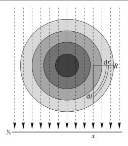
Figure 1. Axial section of a cylindrically symmetric, variable density object. The Abel transform gives the line integral through the object at each point. The infinitesimals are related by  $dl = r dr/\sqrt{r^2 - x^2}$ .
