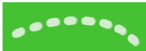
Trajectory of ball, captured at double frame rate, with 50% shutter
