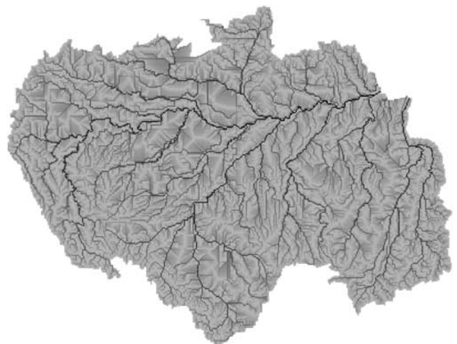
Figure 2. River network. In this figure, the darker the graytone, the higher the drainage area upstream.
