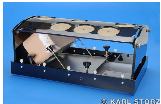
Fig. 5 The hernia model is placed in a quite normal laparoscopic box trainer and closed by a textile membrane that simulates the peritoneum
