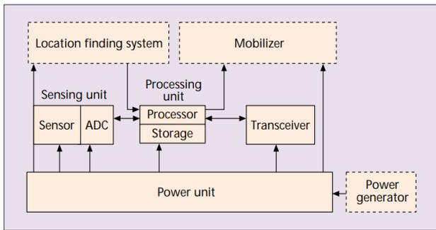
**Figure 2. Hardware components of a sensor node**
