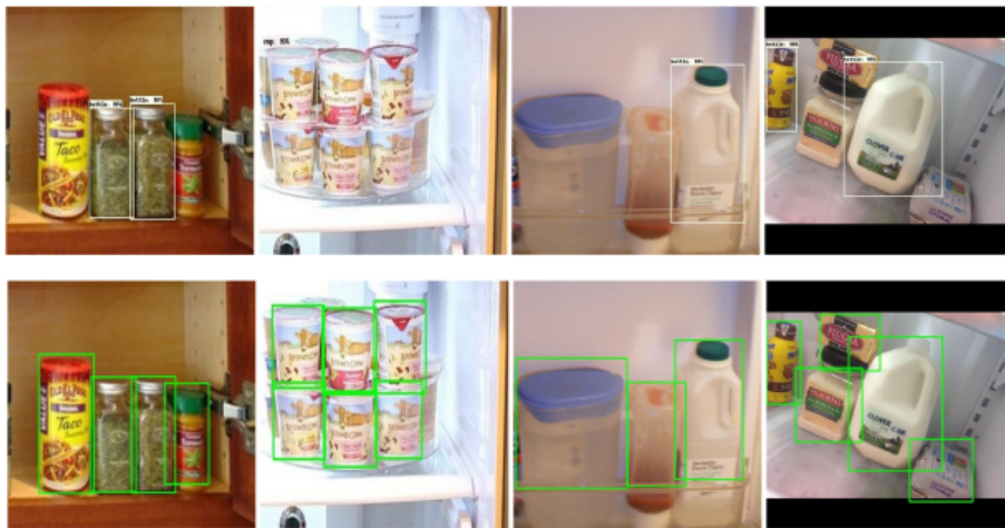
Fig. 4. Figure illustrates the improvement in object detection by finetuning CNN with synthetic rendered dataset. First row highlights the prediction from baseline model trained on COCO dataset with white bound-boxes. Second row marks predictions (with green bound-boxes) from fine-tuned CNN with synthetic dataset.
