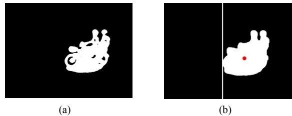
Figure 2. Moving object detection, a) binary extracted moving object, b) closed binary moving object with the detection line and the object centroid
