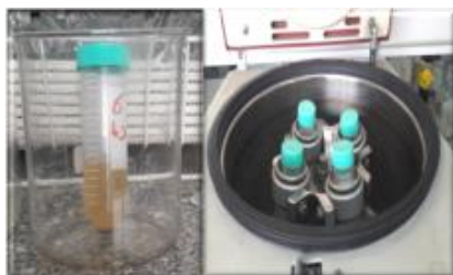
Figure 2. Centrifugation of T.flavus liquid formulations to determine mycelial mass weight
