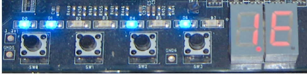
Figure 3.9: LED and seven segment monitoring
