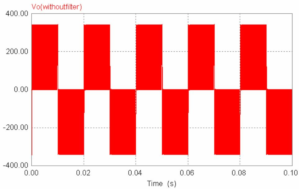
Figure (7.11): Output of the Inverter Without low pass Filter
