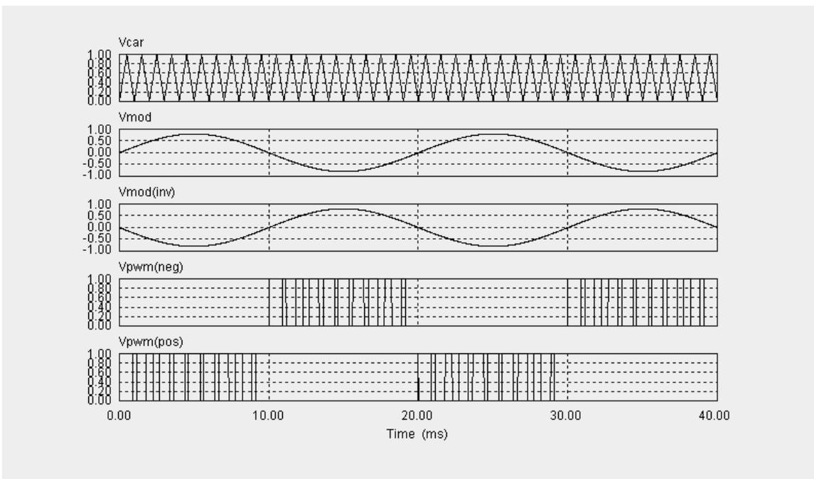
Figure (4.12): Scheme for bipolar & Uni-polar sine pulse width modulation
