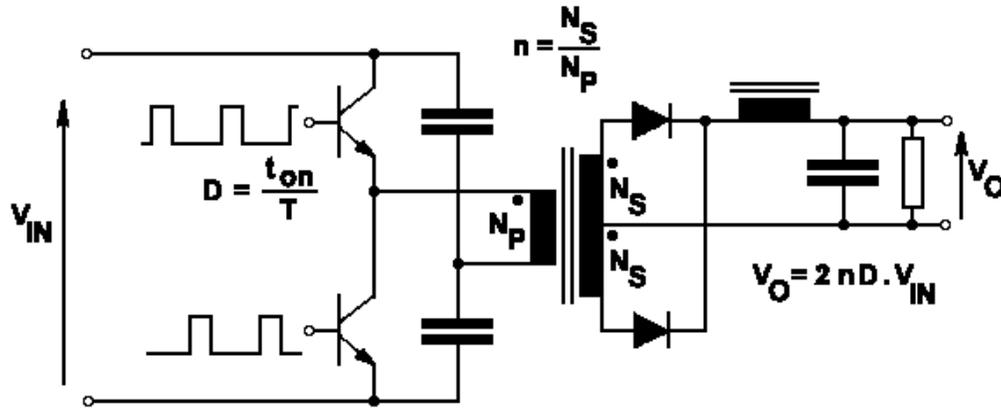
Figure (4.7): Half Bridge Converter
