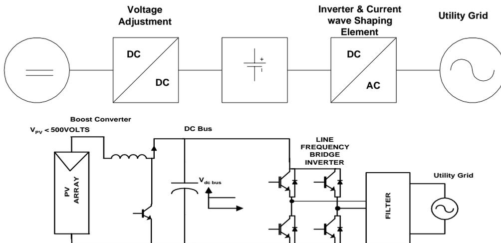
Fig. 3.5 Transformer less PV inverter with several conversion stages including boost stage
