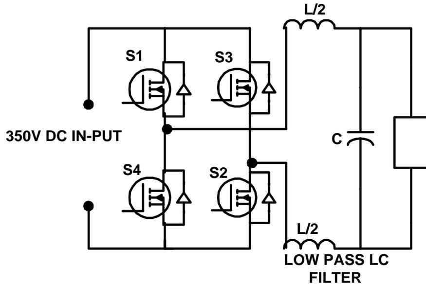
Figure (5.3): basic full bridge topology inverter
