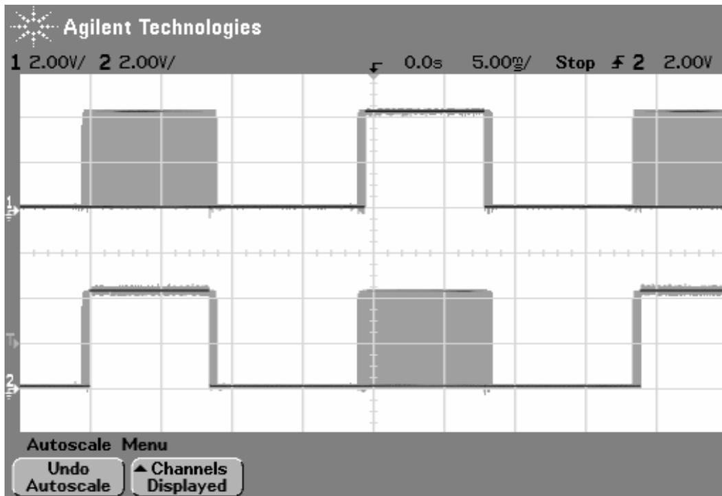
Figure (7.21): Symmetrical HSPWM signals for  $S_3$  &  $S_4$
