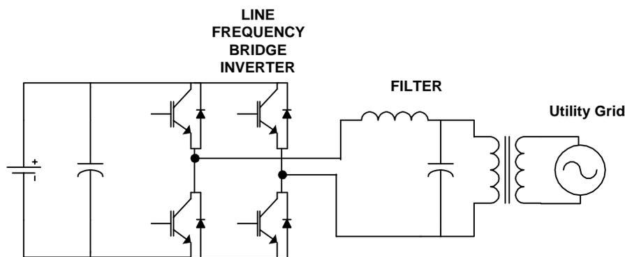
Figure 3.8 Single stage Inverter with line frequency transformer
