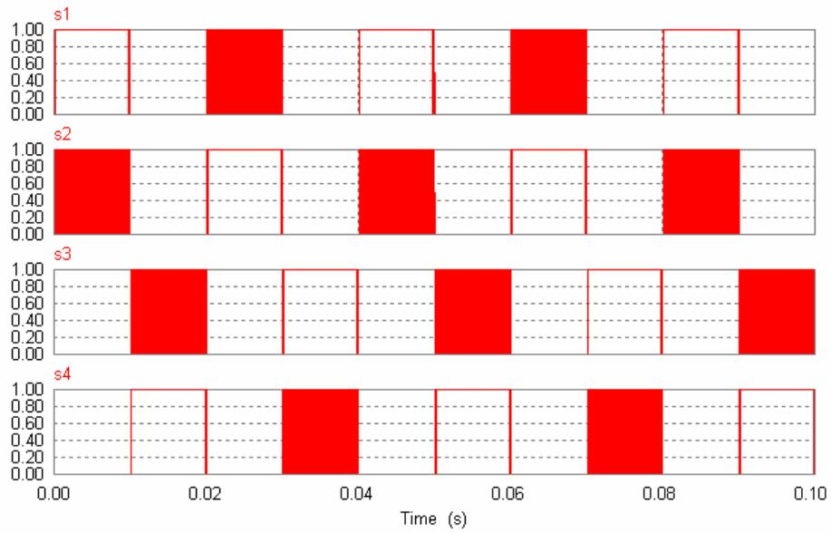
Figure (7.10): Generation of Symmetrical Hybrid Sine PWM signals for the Inverter Switches
