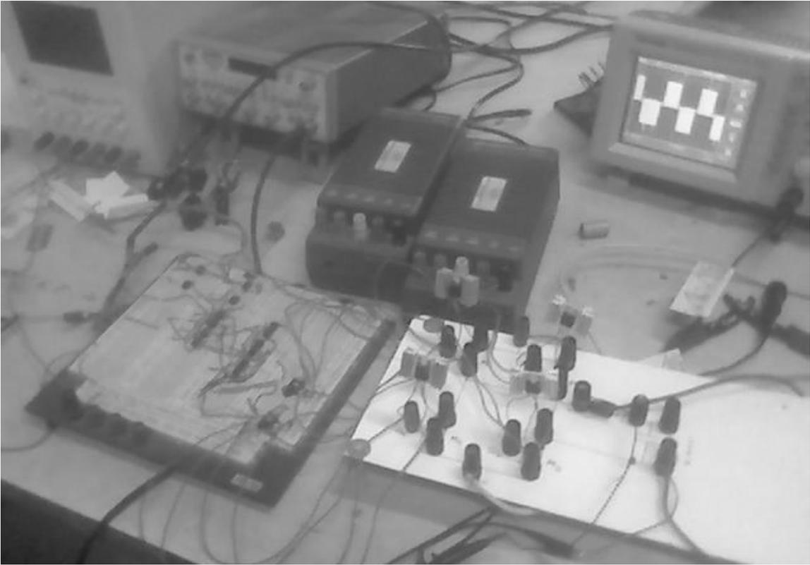
Figure (7.28): Experimental setup for prototype SHSPWM Inverter
