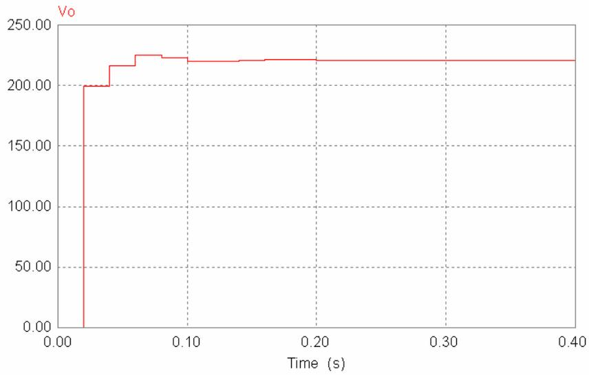
Figure (7.14): Output voltage (RMS) of the Inverter at full load
