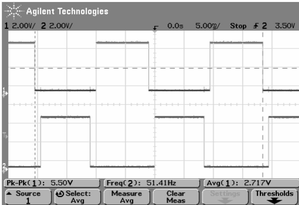
Figure (7.19): Square Wave Signals at line frequency.
