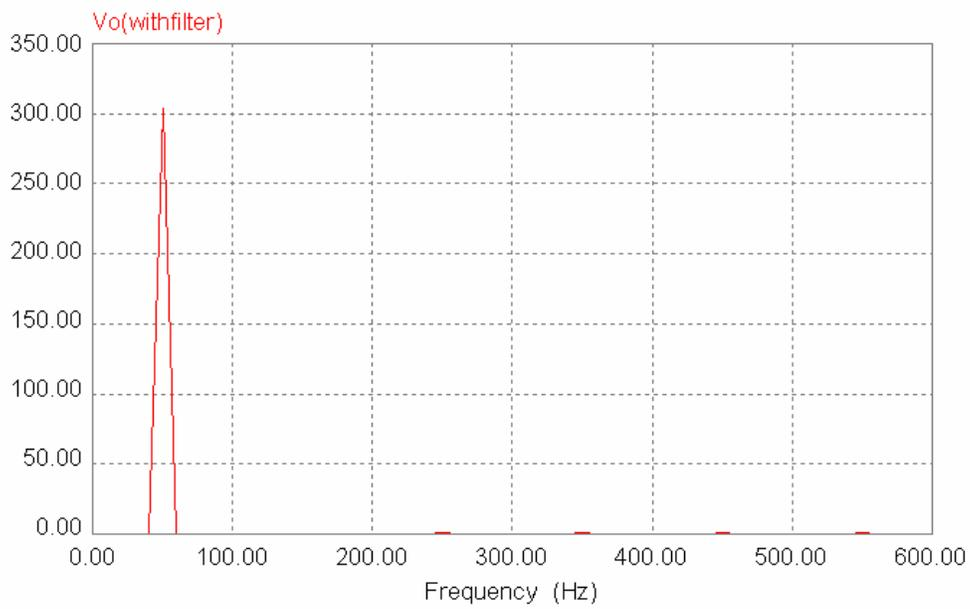
Figure (7.13): FFT for the Inverter output at full load
