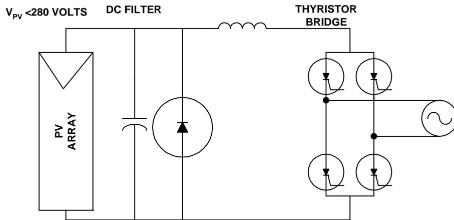
Figure (3.1): Line commutated Transformer less PV inverters
