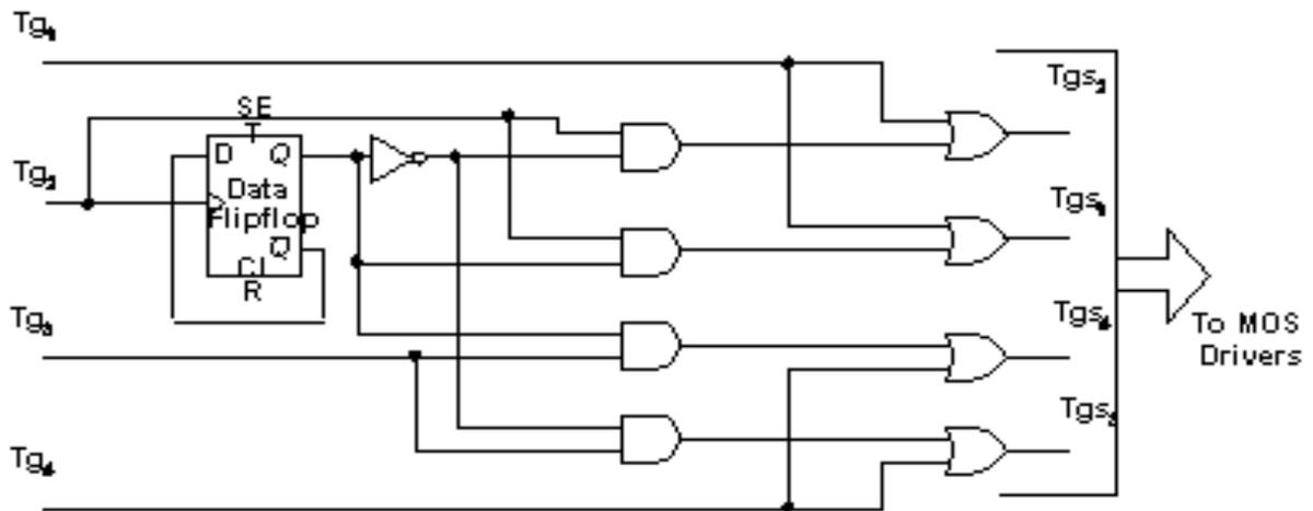
Figure: (5.5) logic circuit for SHSPWM gate signals
