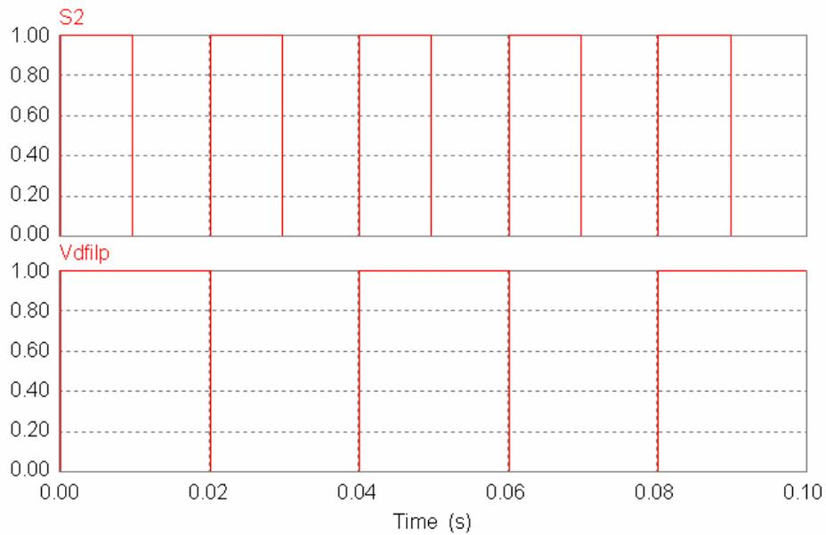
Figure (7.9): Output of the D-Flip-flop (Frequency Divider)
