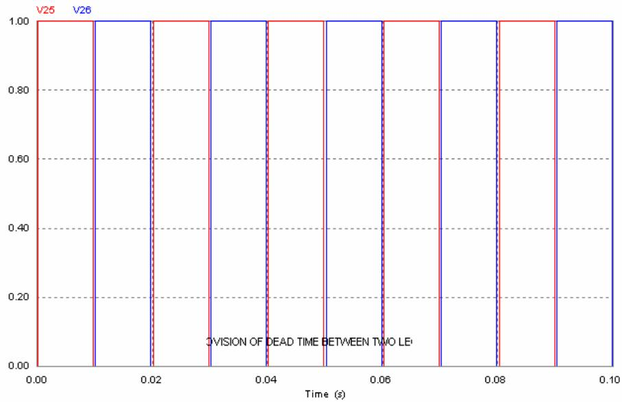
Figure (7.8): Provision of dead time between two switches in each leg.
