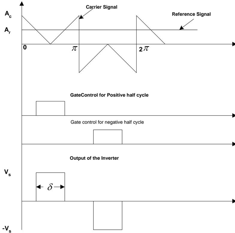
Figure (4.10): Scheme for Single Pulse Width Modulation
