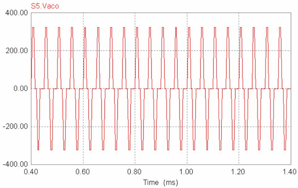
Figure (7.2): Out put of the High frequency switching Transformer
