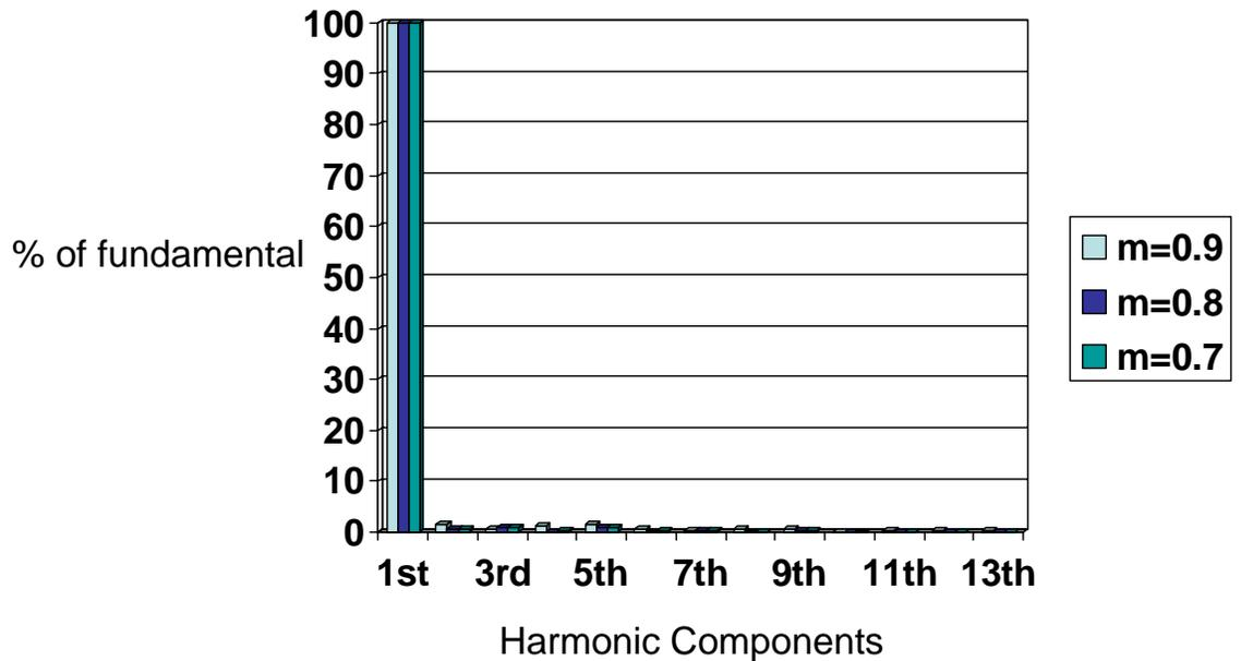
Figure (7.26): % Fundamental Vs Harmonic component for different 'm'.
