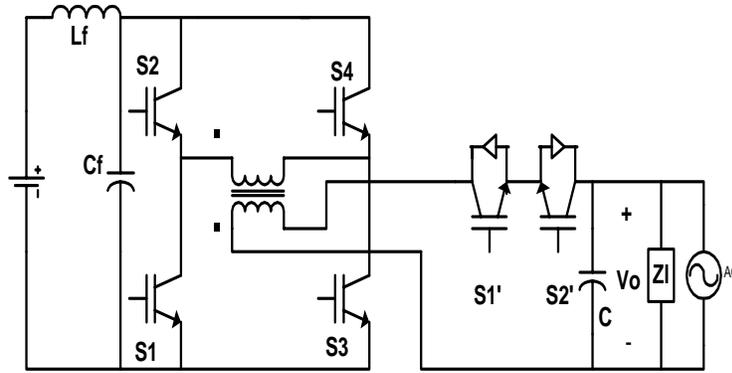
Figure (3.10): Six-switch isolated buck-boost inverter (isolated) by Nagao and Harada
