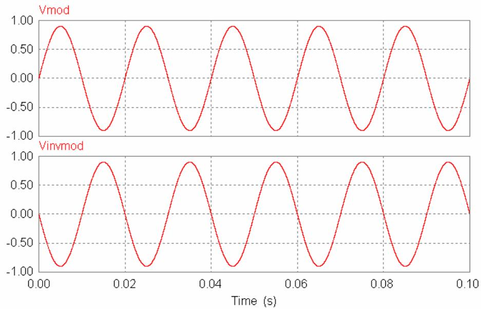
Figure (7.4): Modulating Sine Wave and its Inversion
