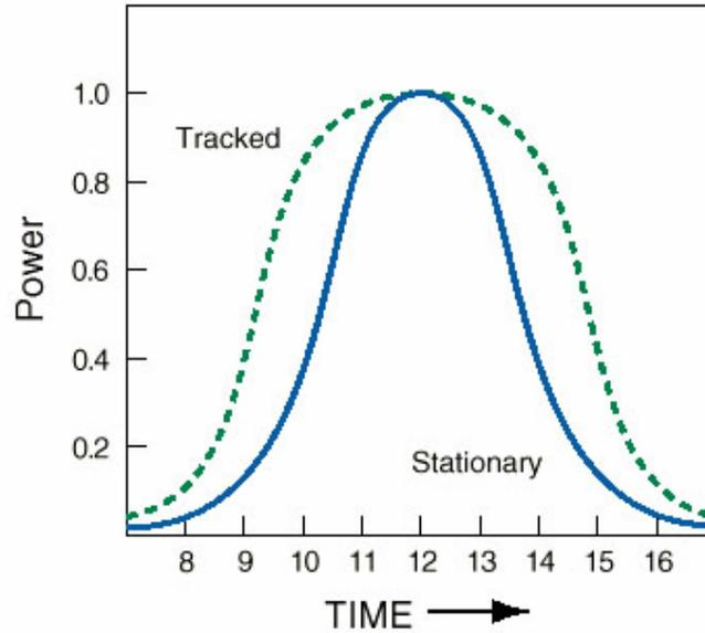
Figure (2.3): The Graph showing power output for tracked and non-tracked array
