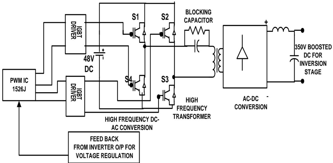
Fig (5.2): schematic for DC-DC converter
