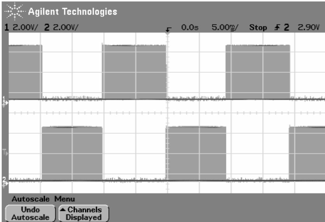
Figure (7.18): Sine PWM Signals
