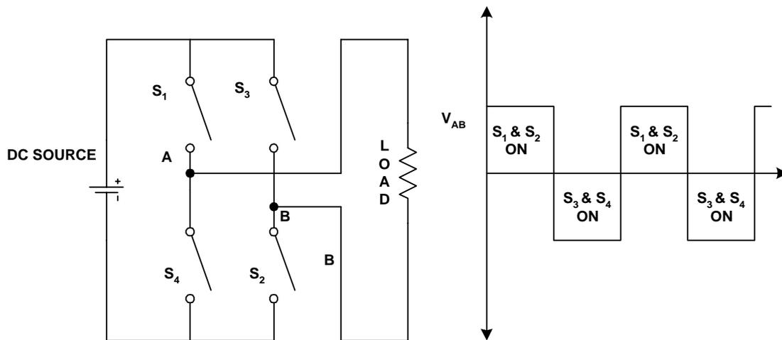
Figure (4.9): Principle of an Inverter Operation
