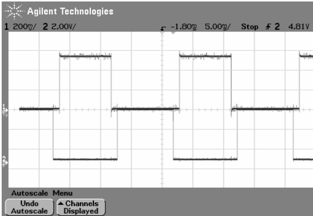
Figure (7.24): Provision of Dead time between two Switches In each leg of the Inverter
