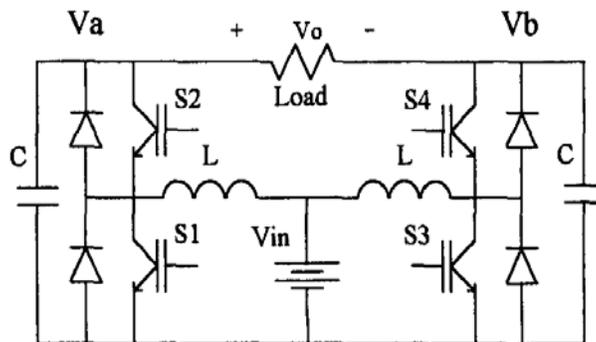
Figure (3.9): Four-switch boost inverter by Cáceres and Barbi [10].
