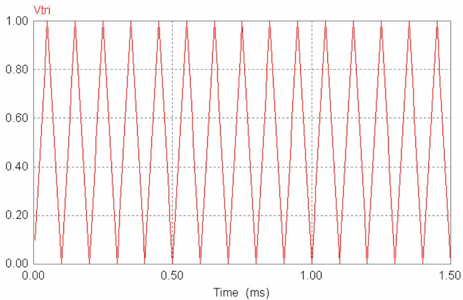
Figure (7.5): Unipolar triangular carrier wave signal
