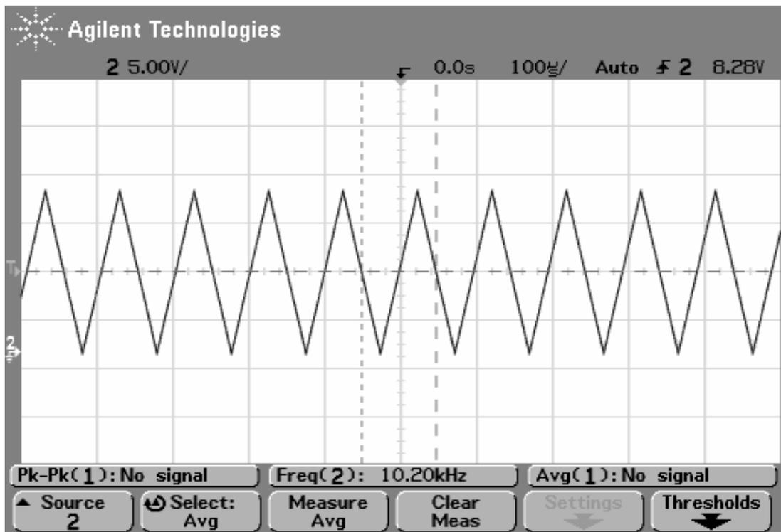
Figure (7.17): Unipolar Triangular Carrier wave
