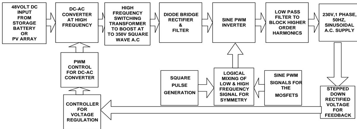
Fig (5.1): Block diagram for the developed inverter
