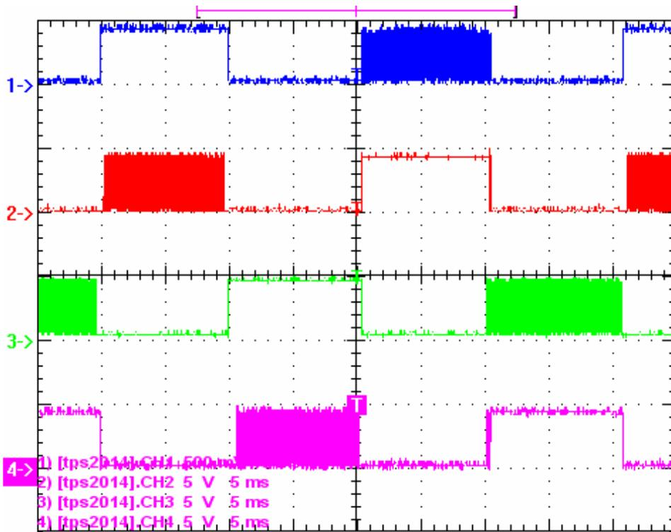
Figure (7.22): SHPWM pulses for switches  $S_1$ ,  $S_2$ ,  $S_3$ , and  $S_4$  respectively (Driver o/p)
