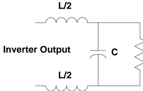
Figure (6.2): Low pass filter for the Inverter
