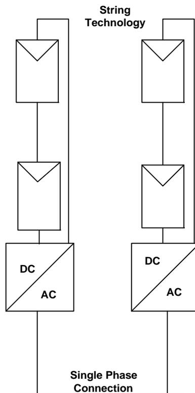
Figure (3.6) Structure of a string inverter
