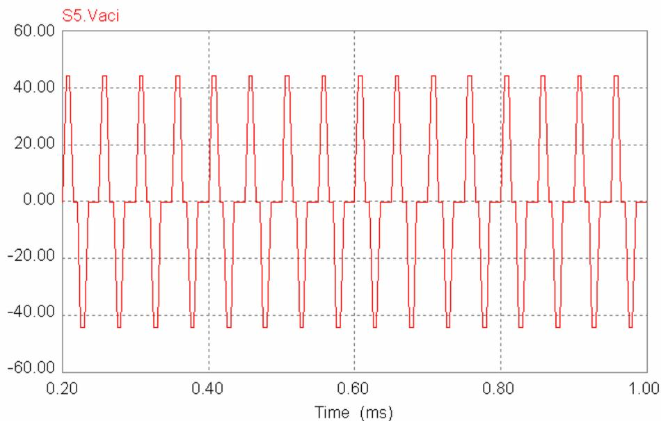
Figure (7.1): Out put of the High frequency Inverter
