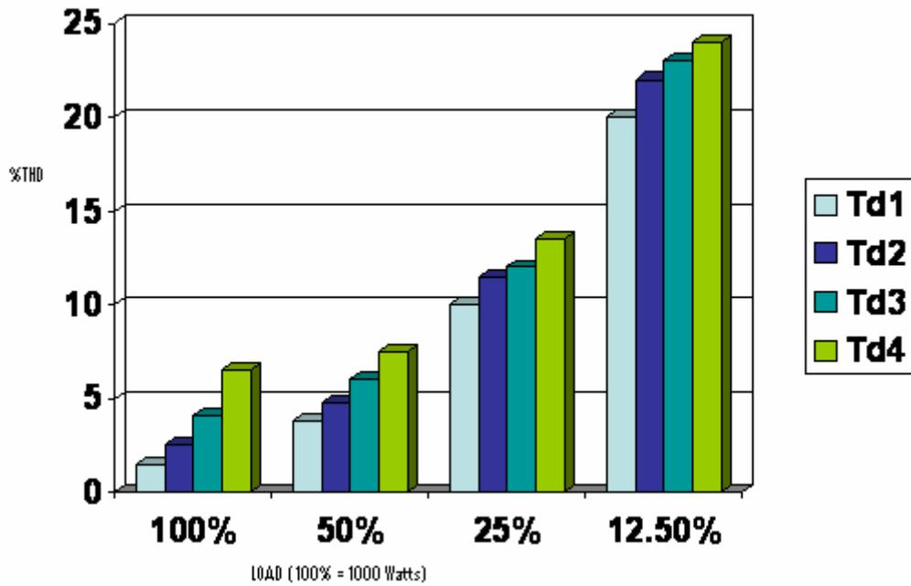
Figure (7.15): THD Verses Load [Td1=0.159ms, Td2=0.318ms, Td3=0.479, Td4=0.641ms]
