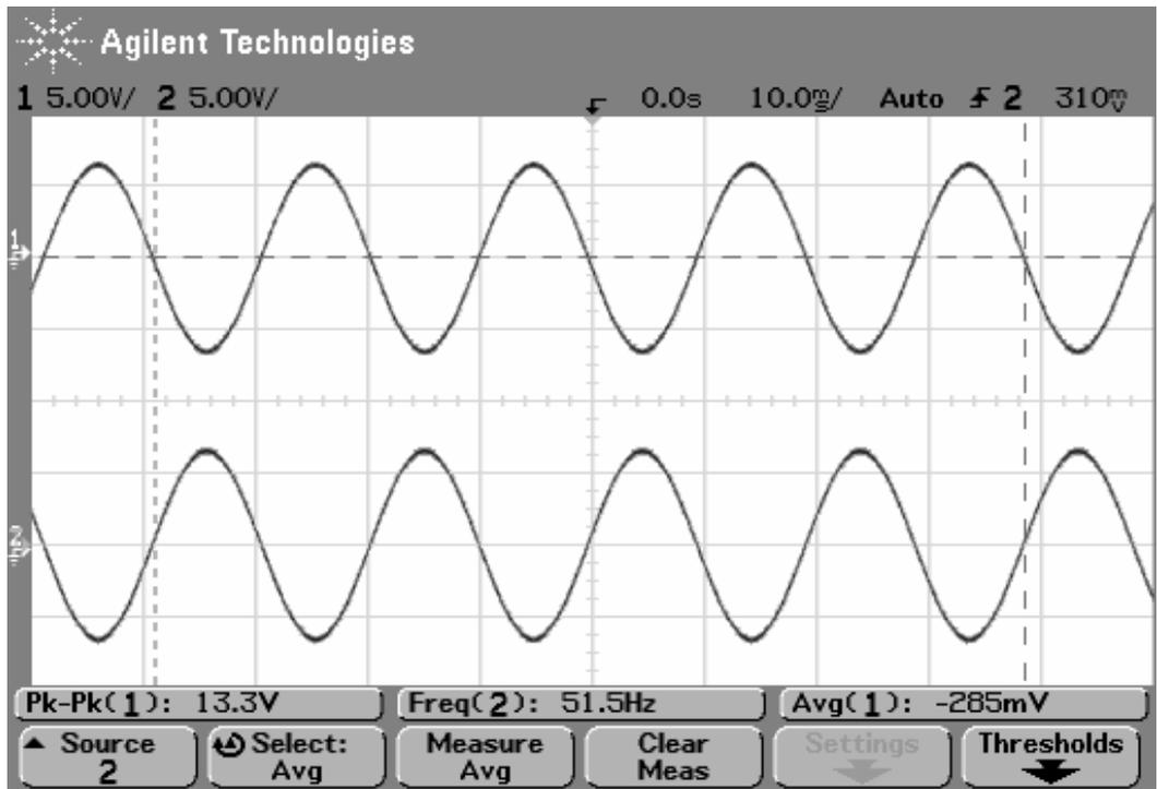
Figure (7.16): Modulating Sine & Inverted Sine Wave
