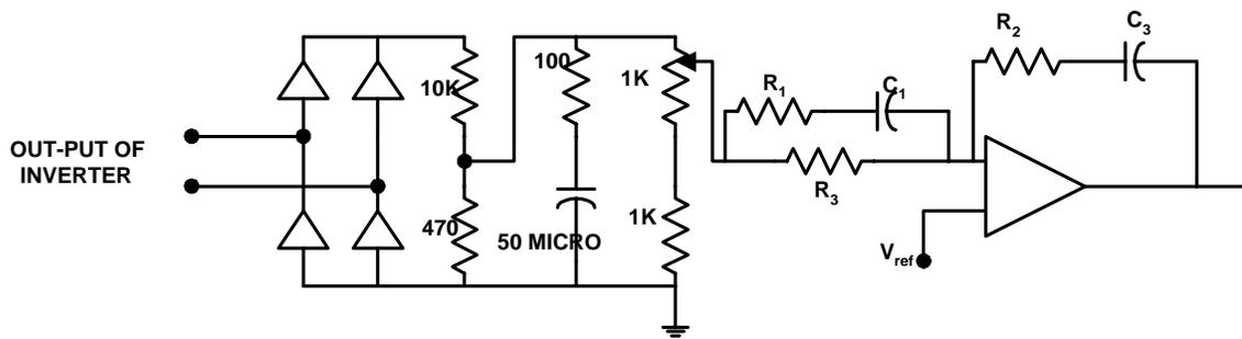
Figure (5.7): Feed Back Circuit & error amplifier for line regulation
