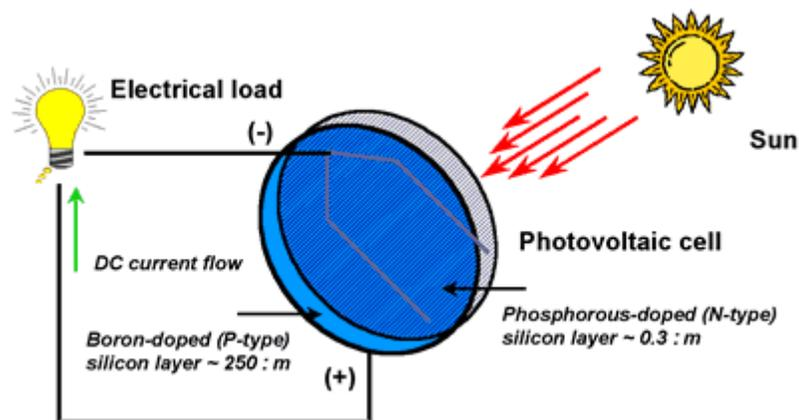
Figure: 2.1 Operation of photovoltaic cell.
