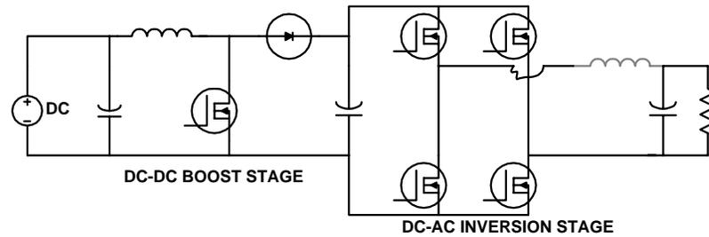
Figure (3.11): Two-stage boost inverter [9].
