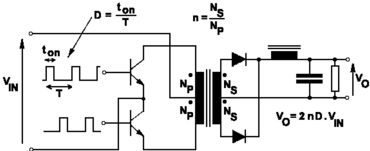
Figure (4.6): Push-Pull Converter
