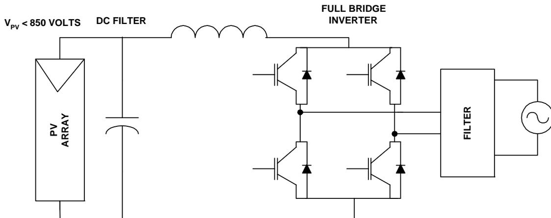
Figure (3.2): Self commutated inverters with out transformer
