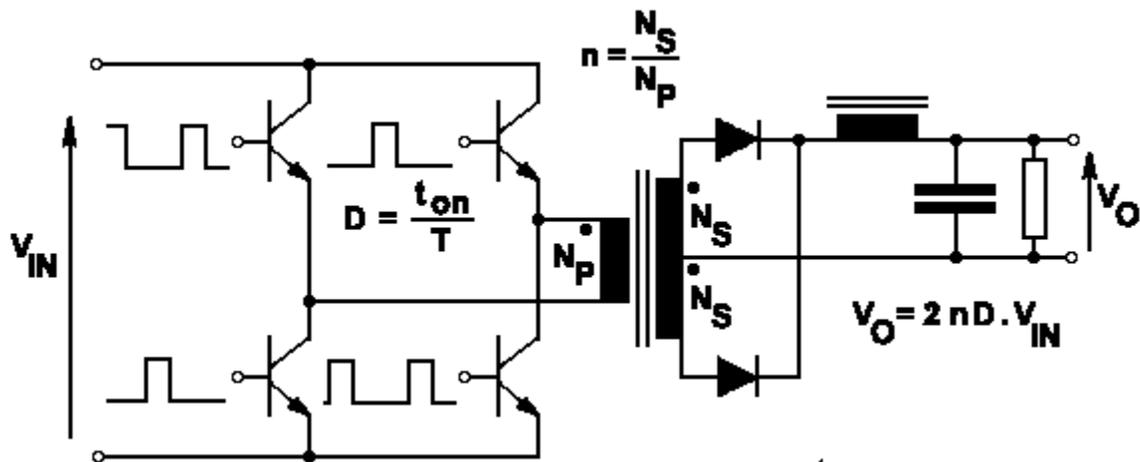
Figure (4.8): Full Bridge Converter
