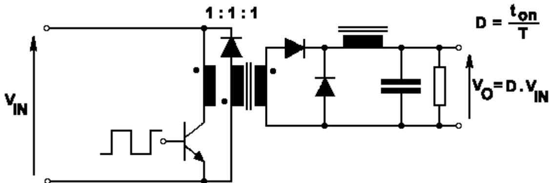
Figure (4.5): Forward Converter
