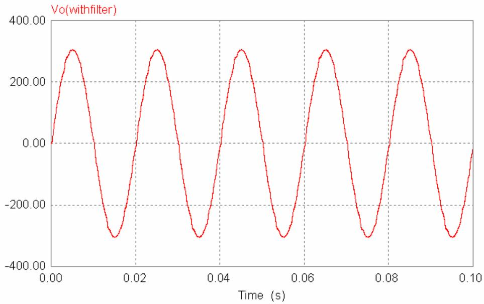
Figure (7.12): Output of the Inverter With low pass Filter at full load
