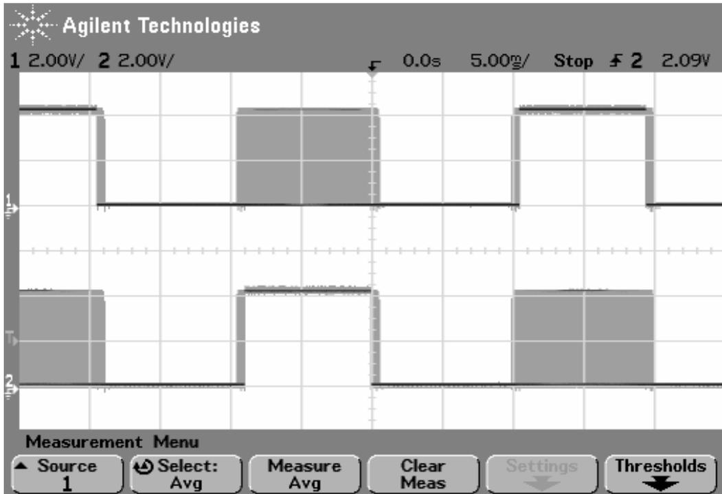
Figure (7.20): Symmetrical HSPWM signals for  $S_1$  &  $S_2$
