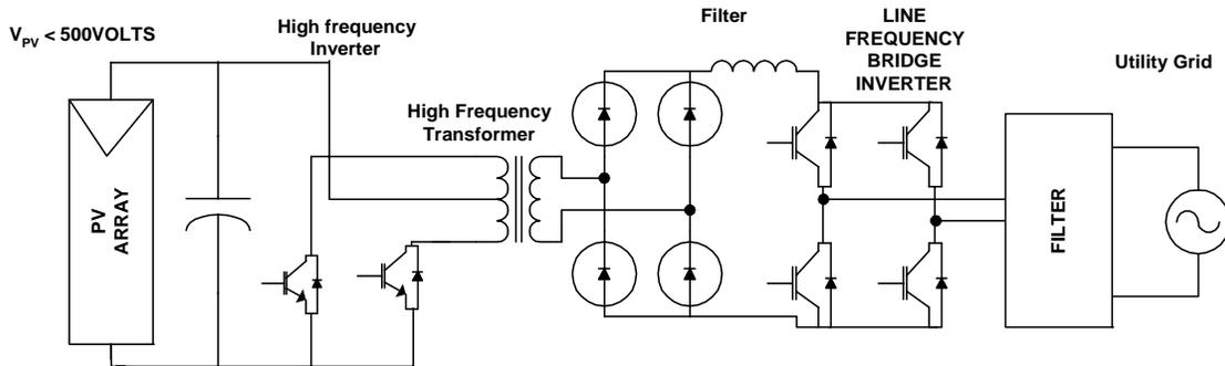
Fig: (3.4) PV inverter with several conversion stages and high frequency transformer
