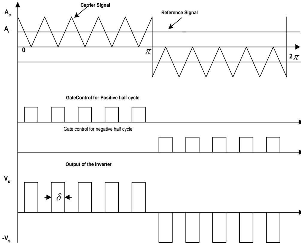
Figure (4.11): Scheme for multiple pulse width modulation
