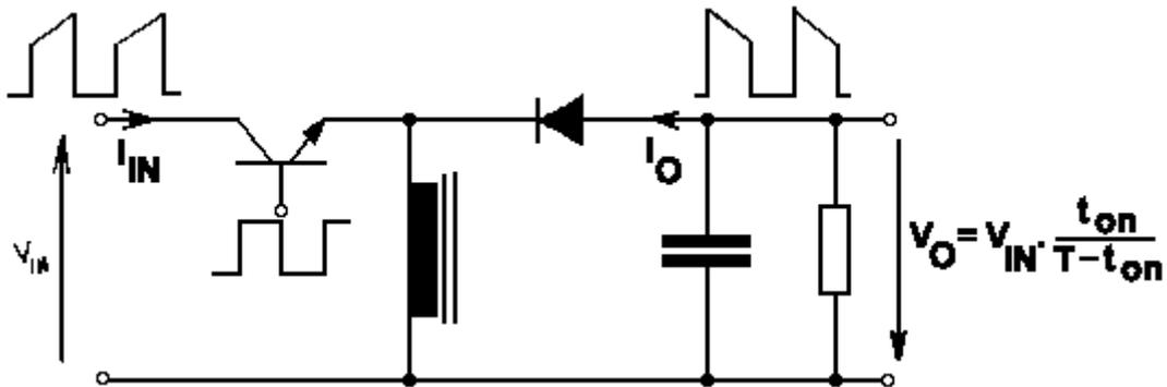
Fig (4.3): Buck-Boost Converter
