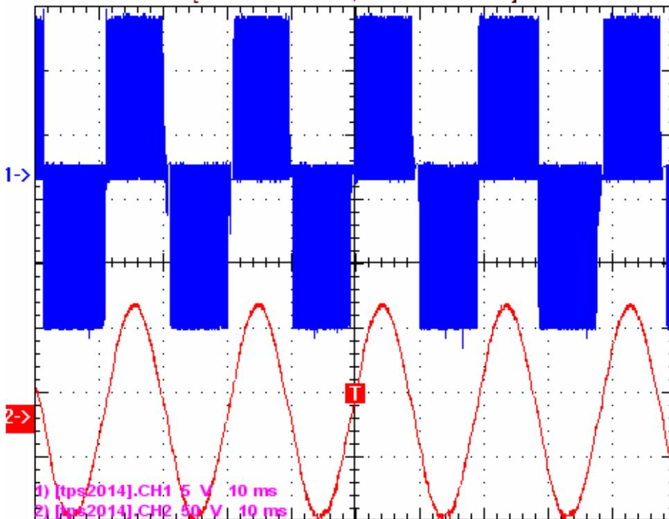
Figure (7.23): Out put of Inverter with and with out low pass filter
