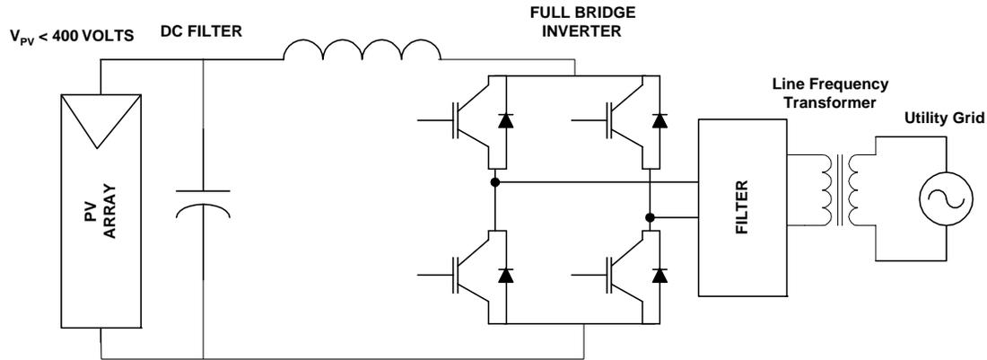
Figure (3.3): PV inverters with line frequency transformer
