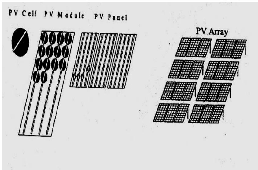
Figure (2.2): PV cell, PV module, PV panel, PV Array
