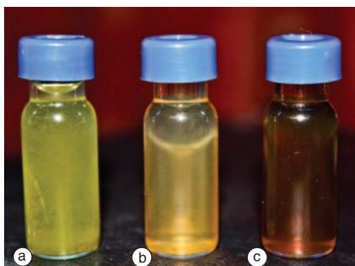
Fig. 1. Formation of AgNPs using Cynodon dactylon leaf extract: (a) Cynodon dactylon grass leaf extract (yellow); (b) Silver nitrate solution with Cynodon dactylon grass leaf extract at 0 mins (yellowish-brown); and (c) Formation of AgNPs after 20 mins of mixing (dark brown).
