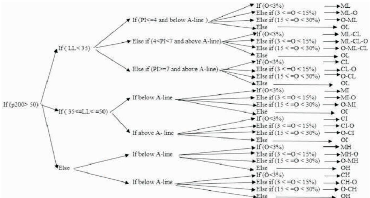
Figure 1. Algorithm for ISC Classification System
