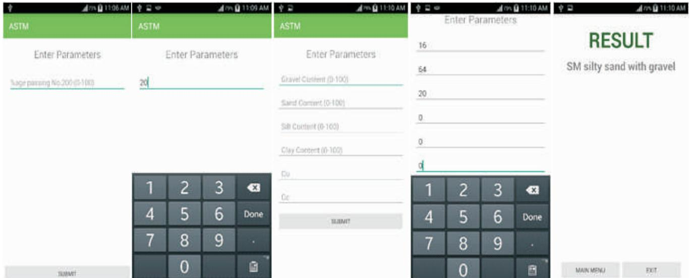
Figure 8. Soil Classification for Soil B using Mobile App and ASTM System of Soil Classification (after Kumar et al. (2015))
