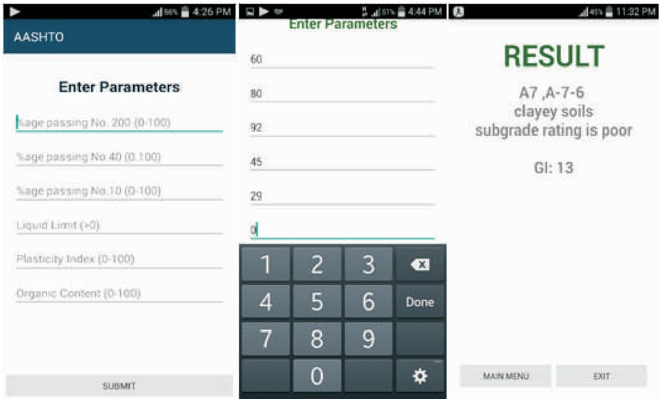
Figure 6. Soil Classification Using Mobile App (AASHTO System)
