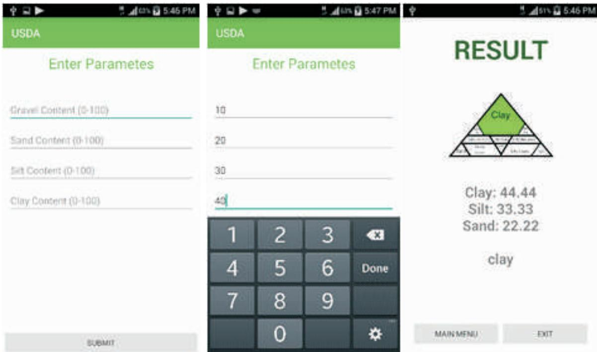
Figure 5. Soil Classification using Mobile App (USDA System)
