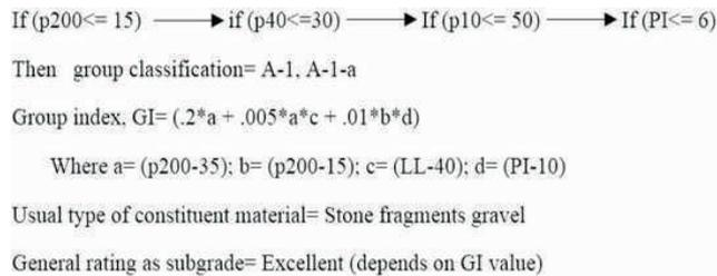
Figure 4. Sample Algorithm for AASHTO Classification System
