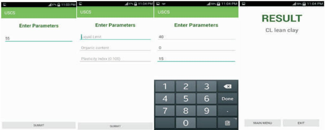
Figure 10. Soil Classification using Mobile App (USCS System)
