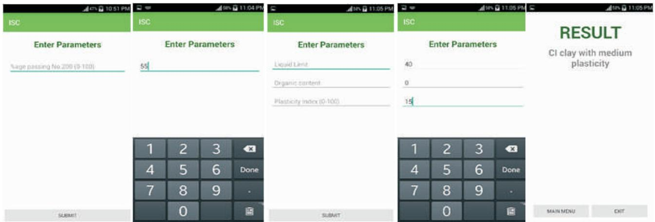
Figure 11. Soil Classification using Mobile App (ISC System)
