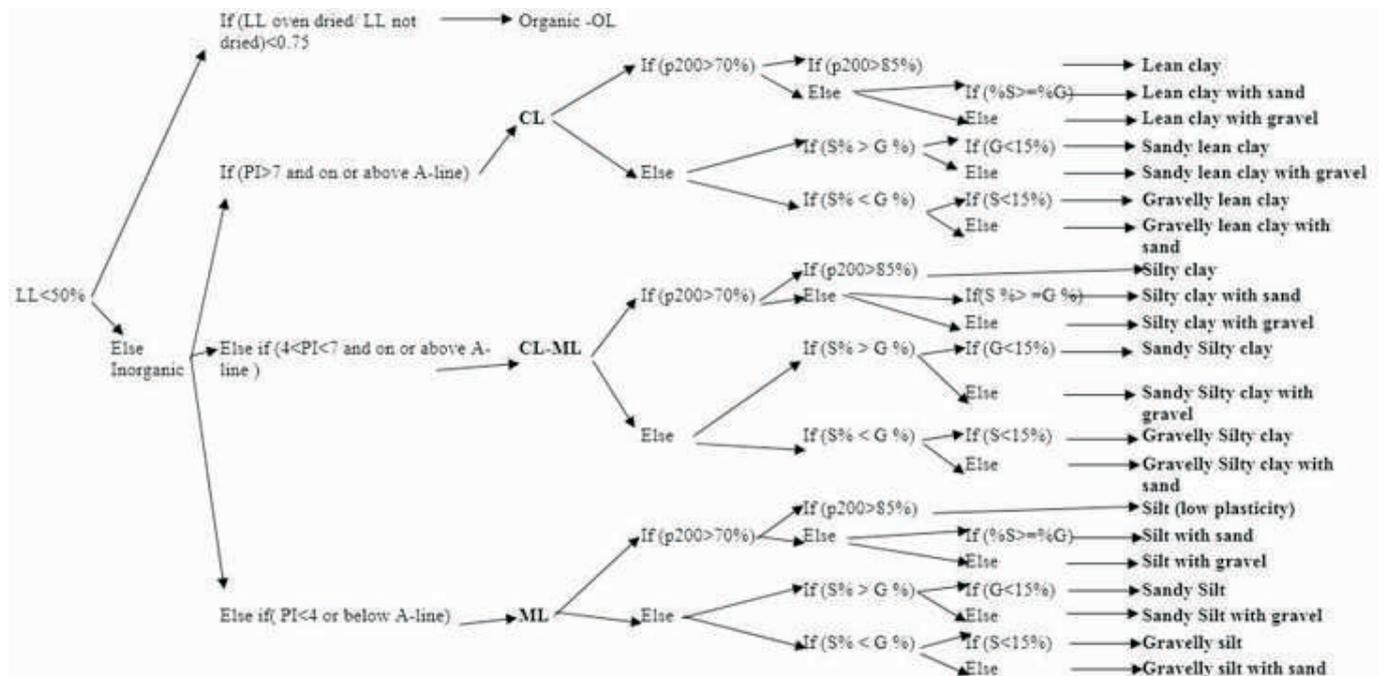
Figure 2. Algorithm for ASTM Classification System
