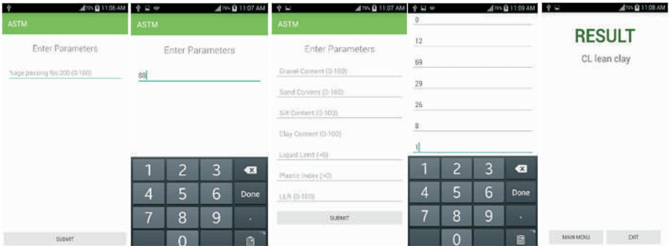
Figure 7. Soil Classification for Soil a using Mobile App and ASTM System of Soil Classification (after Kumar et al. (2015))
