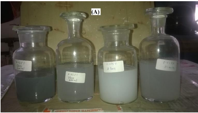
Figure 5 (A) & (B) Shows comparison between nanofluid sedimentation containing 0.015% ( by vol.) nanoparticle at different sonication time(30 min, 2 hr, 3 hr, 5 hr from right). (A) just after sonication. (B) after 25 hr of sonication.
