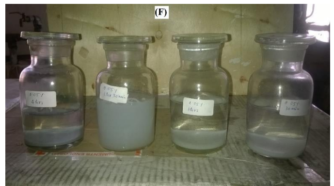
Figure 5 (E) & (F) Shows comparison between nanofluid sedimentation containing 0.05% ( by vol.) nanoparticle at different sonication time(30 min, 1 hr, 1hr 30 min, 5 hr from right). (E) just after sonication. (F) after 25 hr of sonication.
