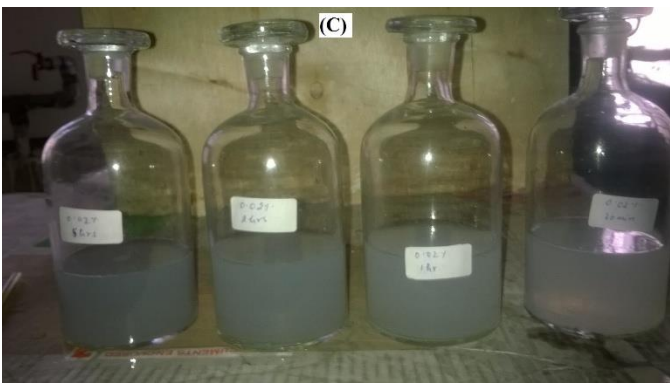
Figure 5 (C) & (D) Shows comparison between nanofluid sedimentation containing 0.02% ( by vol.) nanoparticle at different sonication time(30 min, 1 hr, 2 hr, 5 hr from right). (C) just after sonication. (D) after 25 hr of sonication.
