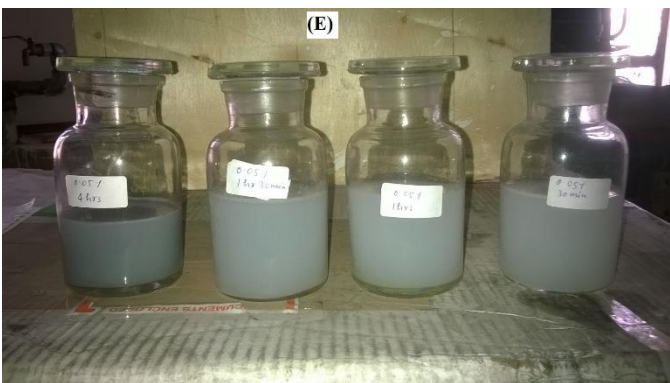
Figure 5 (E) & (F) Shows comparison between nanofluid sedimentation containing 0.05% ( by vol.) nanoparticle at different sonication time(30 min, 1 hr, 1hr 30 min, 5 hr from right). (E) just after sonication. (F) after 25 hr of sonication.
