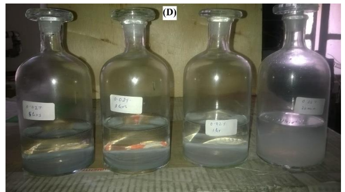
Figure 5 (C) & (D) Shows comparison between nanofluid sedimentation containing 0.02% ( by vol.) nanoparticle at different sonication time(30 min, 1 hr, 2 hr, 5 hr from right). (C) just after sonication. (D) after 25 hr of sonication.
