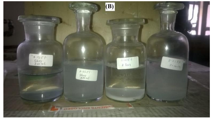
Figure 5 (A) & (B) Shows comparison between nanofluid sedimentation containing 0.015% ( by vol.) nanoparticle at different sonication time(30 min, 2 hr, 3 hr, 5 hr from right). (A) just after sonication. (B) after 25 hr of sonication.
