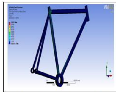
Figure 20: Equivalent stress, Steady state pedaling
