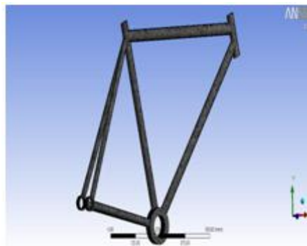
Figure 3: Bike frame with meshing of 5mm
