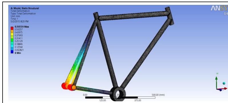
Figure 28: Rear wheel braking (maximum deformation), Aluminum 6061-T
