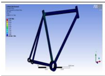
Figure 21: Equivalent stress, Vertical impact
