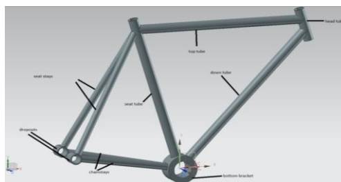
Figure 1: Tubing diagram of the bike frame
