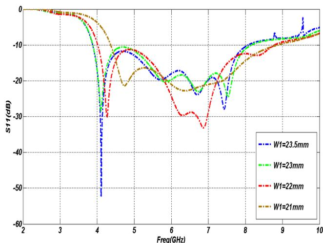
**Figure 4.** The Return loss of the antenna for various values of patch diameter,  $W_1$ .  $W_2 = 11.5$  mm,  $P = 5$  mm,  $H = 8$  mm,  $X = 5.7$  mm,  $X_1 = 4.5$  mm,  $X_2 = 2$  mm,  $Y_1 = 4$  mm,  $Y_2 = 8$  mm and  $R = 1.5$  mm.
