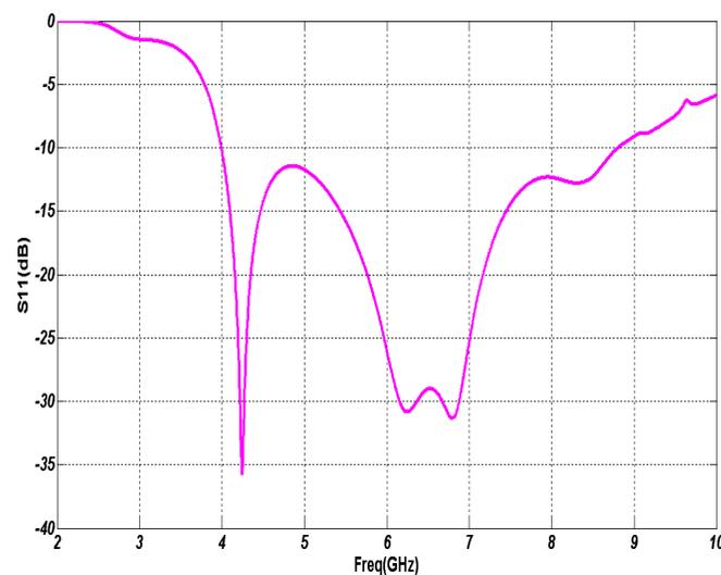
Figure 3. Return loss of the proposed antenna.  $W_1 = 22$  mm,  $W_2 = 11.5$  mm,  $P = 5$  mm,  $H = 8$  mm,  $X = 5.7$  mm,  $X_1 = 4.5$  mm,  $X_2 = 2$  mm,  $Y_1 = 4$  mm,  $Y_2 = 8$  mm and  $R = 1.5$  mm.
