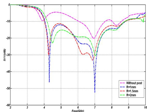
**Figure 5.** Return Loss of the antenna for various diameters of the posts.  $W_1 = 22$  mm,  $W_2 = 11.5$  mm,  $P = 5$  mm,  $H = 8$  mm,  $X = 5.7$  mm,  $X_1 = 4.5$  mm,  $X_2 = 2$  mm,  $Y_1 = 4$  mm,  $Y_2 = 8$  mm.
