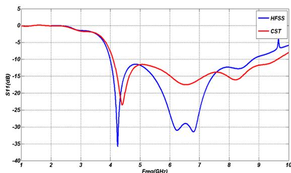
**Figure 6.** Comparison of the S11 obtained through HFSS and CST.  $W_1 = 22$  mm,  $W_2 = 11.5$  mm,  $P = 5$  mm,  $H = 8$  mm,  $X = 5.7$  mm,  $X_1 = 4.5$  mm,  $X_2 = 2$  mm,  $Y_1 = 4$  mm,  $Y_2 = 8$  mm and  $R = 1.5$  mm.
