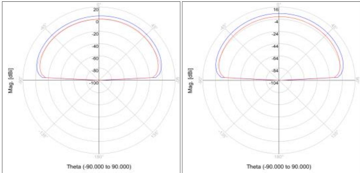
**Fig 5:** E & H- Field of 10 GHz antenna on fr-4 substrate
