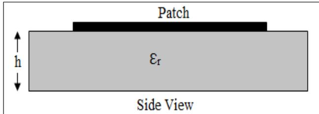
Fig 2: Geometry of the microstrip patch antenna
