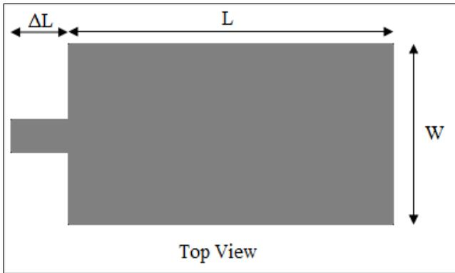
Fig 1: Top view of microstrip
