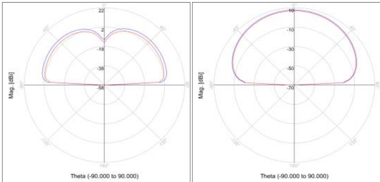
**Fig 6:** E & H- Field of 900 MHz antenna on rogers-5880 substrate
