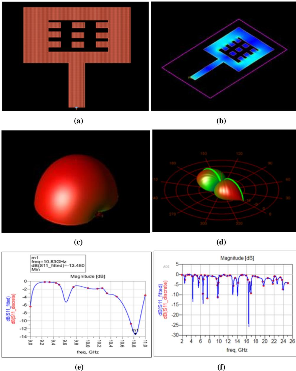
**Fig 1:** (a) Layout of fractal notch in a simple strip antenna, (b) 3D layout of fractal notch in a simple strip antenna, (c) Radiation pattern of non-fractal notch antenna, (d) Radiation pattern of fractal patch antenna, (e) Return loss for non-fractal notch antenna, (f) Return loss for non-fractal notch antenna
