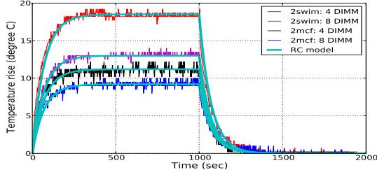
**Figure 4. DIMM's transient temperature (referenced to idle temperature)**
