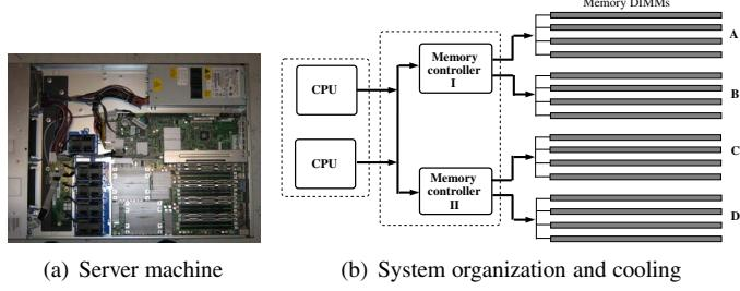
**Figure 1. Intel dual socket Xeon server**
