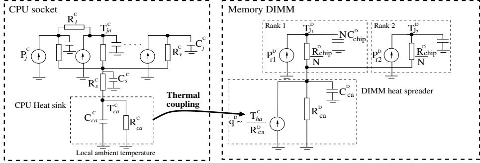
**Figure 2. Combined thermal model**
