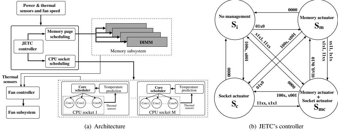
**Figure 8. Architecture and controller of JETC. Each edge denotes a transition annotated with a compound condition of 4 bits. Bit-1 (LSB) is true when CPU’s temperature is high. Bit-2 is true when memory temperature is high. Bit-3 is true when the number of active DIMMs is larger than the default value. Bit-4 is true when there is a fan speed imbalance. The x-mark denotes a don’t care.**
