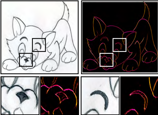
Figure 5: An advantage of the second derivative mask is that it allows detecting the boundary line of the filled primitive. Yellow color represents component x that corresponds to dx mask and pink color y component that corresponds to dy .
