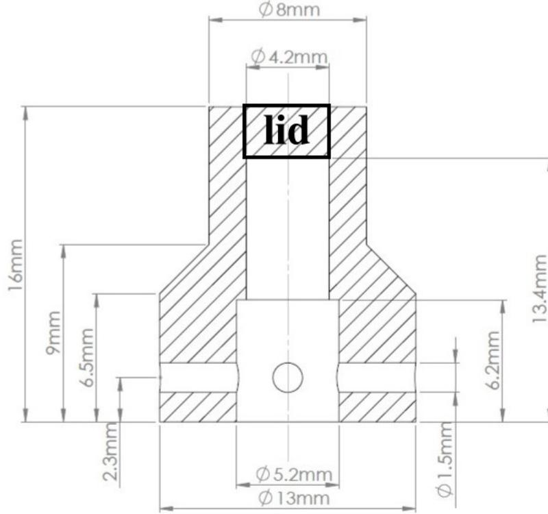
Figure 2: Modelling the metallic core geometry using the *SolidWorks* software.
