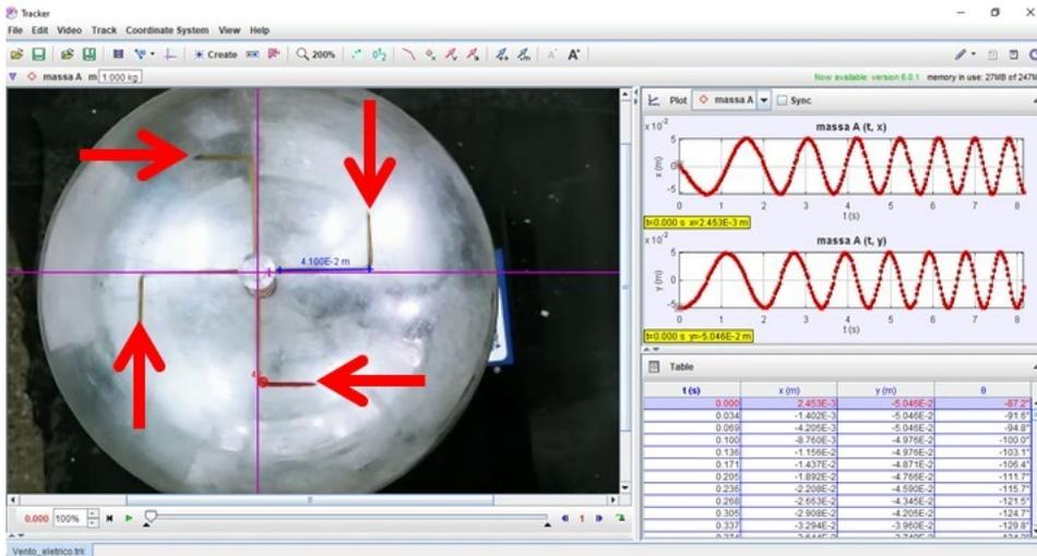
Figure 1: Experimental apparatus. (a) Electric whirl fabricated by brazilian company Azeheb of instruments for physics didactic laboratories. (b) Electric whirl separated in its different metallic parts: core + 4 arms. (c) Smartphone recording the rotation movement of electric whirl on the top of the electrostatic generator. (d) Video analysis process result using the *Tracker* software.
