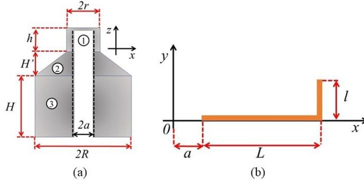
Figure 3: Modelling the geometry of the electric whirl. (a) Core modelled in terms of truncated cone between two cylinders, with lengths given by  $H = 0.65 \text{ cm}$ ,  $H' = 0.25 \text{ cm}$ ,  $h = 0.7 \text{ cm}$ ,  $r = 0.4 \text{ cm}$ ,  $a = 0.26 \text{ cm}$  and  $R = 0.65 \text{ cm}$ . (b) Arms with lengths  $L = 4 \text{ cm}$  and  $l = 2.1 \text{ cm}$ . (c) *SolidWorks* simulation.
