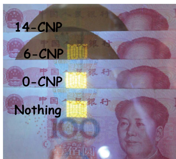
Fig. 9 UV-blocking performance of CNP samples. Paper money was shielded by nothing, 0-CNP, 10-CNP and 14-CNP, respectively, and then exposed to UV light (LED, 10 cm in height, wavenumber of 365 nm).
