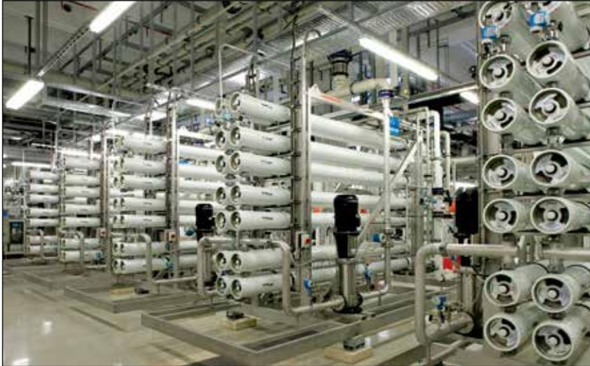
complete biological treatment and the retention of pathogens including viruses has become possible; treatment with membrane bioreactor produces a highly clarified effluent that can be more easily disinfected. Thus treatment with MBR followed by RO and UV treatment is ideal for producing non-potable water.
