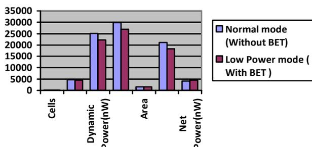
Fig. 6: Generated bar-graph indicating power consumption details of the design in two modes (normal and low power modes)
