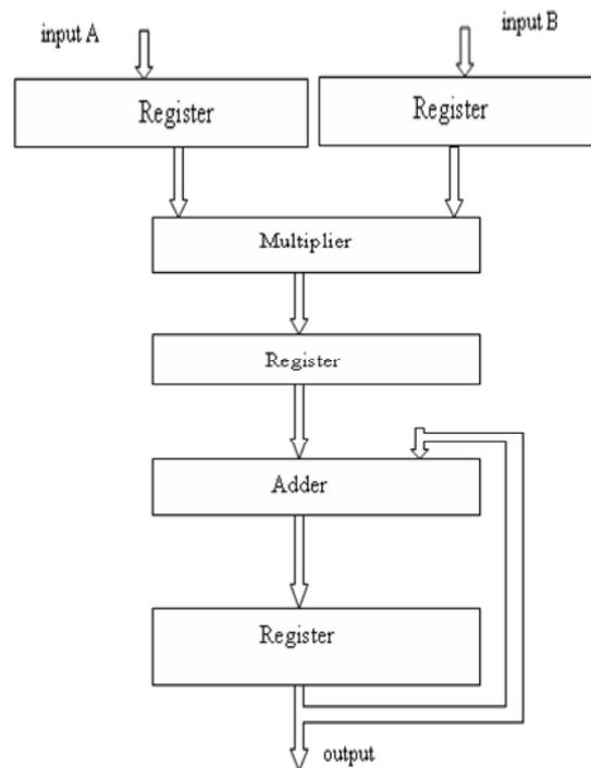
**Fig 4:** General Block Diagram of a Pipeline MAC with block enabling Technique cs - control signal
