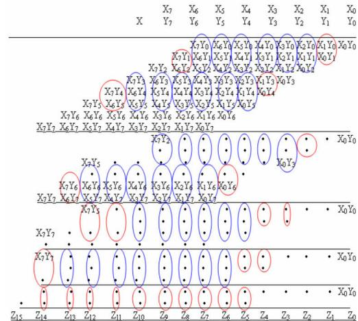
Fig 3: Algorithm for 8 bits x 8 bits Wallace tree multiplier (Harun, 2007)
