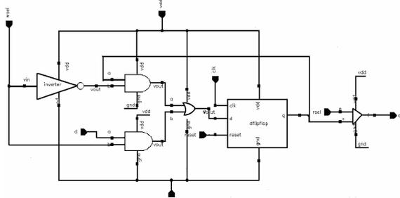
Fig 6: 1 bit Register cell
