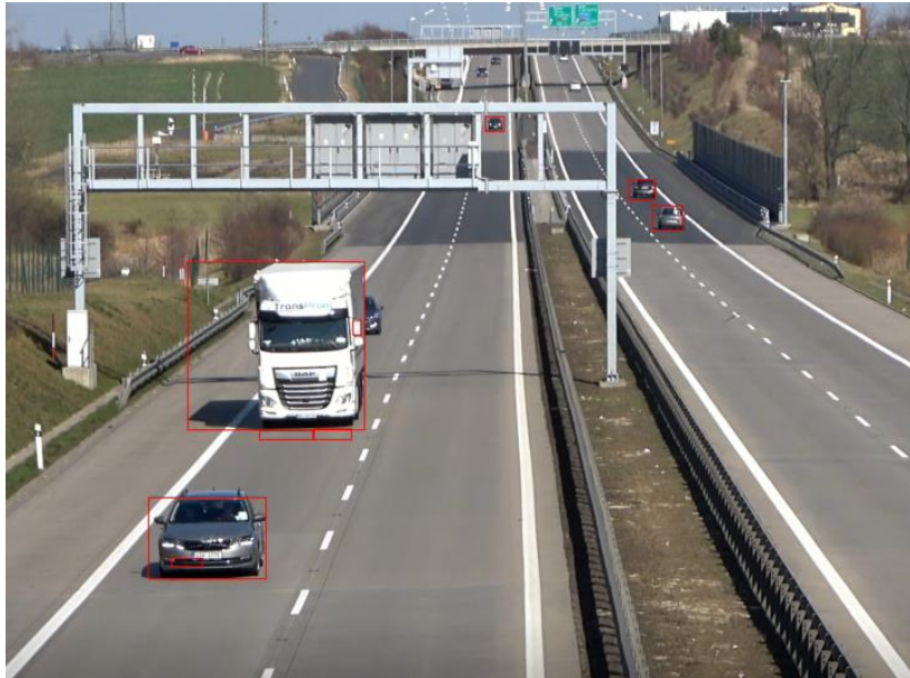
Figure 35 Result of the Object Detection and Tracking for Vehicles in the Afternoon with the Objects Moving in two directions (Bidirectional) [Sample Video 1]
