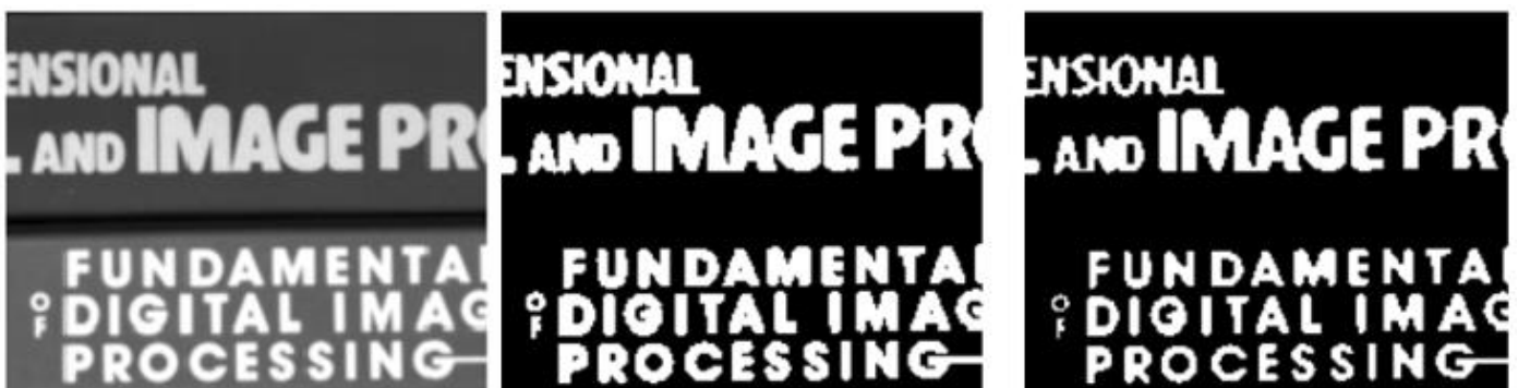
Figure 15 (left) The Grayscale Image, (middle) the Binary Image by Thresholding, (right) Erosion of an Image (Efford, 2000)
