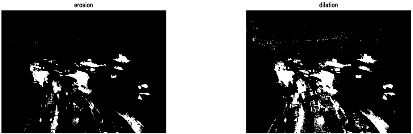
Figure 68 The Erode Morphological Operation (left), the Dilate Morphological Operation (right) of the Sample Video 3
