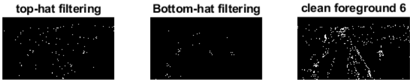
Figure 6 The Top-hat Morphological Operation (left), the Bottom-hat Morphological Operation (middle), the Morphological Operation obtained by subtracting Dilate and Erode (from Figure 5)
