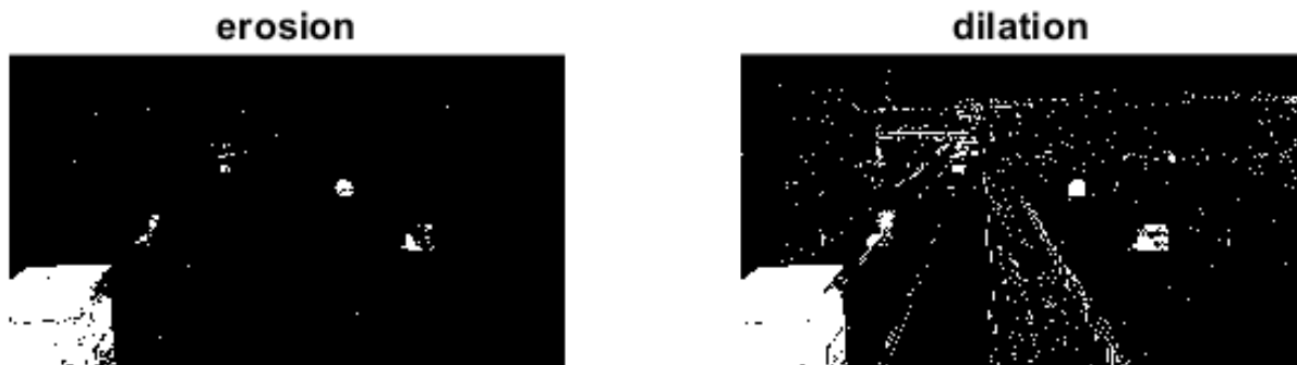
Figure 5 The Erode Morphological Operation (left), the Dilate Morphological Operation (right)
