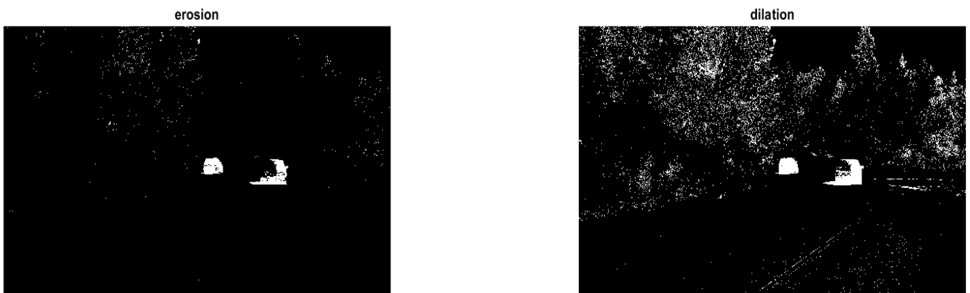
Figure 64 The Erode Morphological Operation (left), the Dilate Morphological Operation (right) of the Sample Video 2
