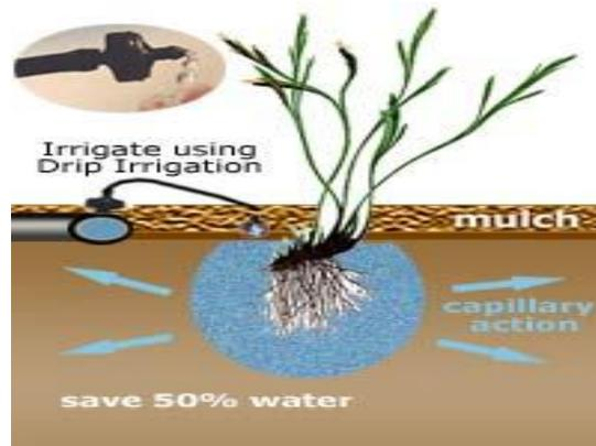
**Figure 2: Drip Irrigation**
