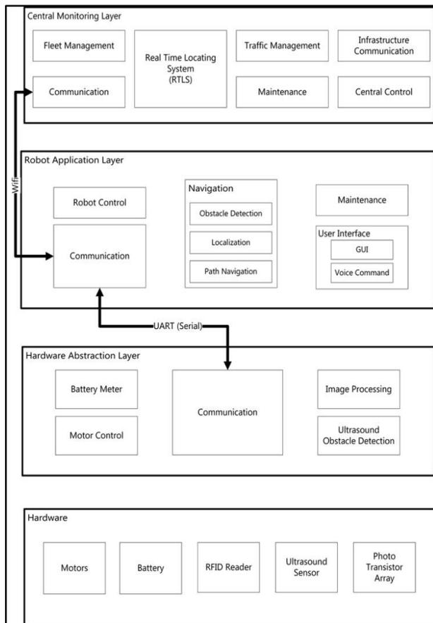
Fig. 2. Layered Architecture of the Entire System
