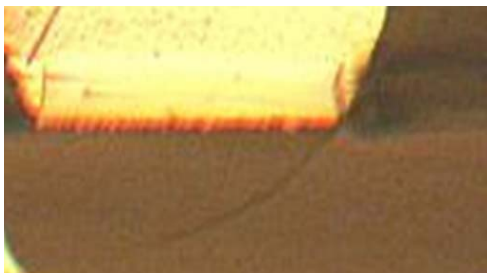
Figure 12: Partial pad crater on PCB side.
