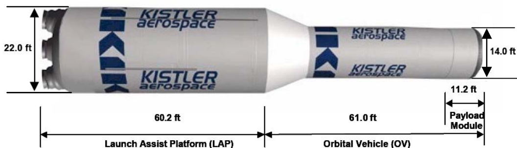
Figure 9. K-1 vehicle profile. (Reprinted with permission of Rocketplane Kistler, Inc).
