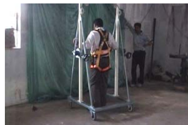
Fig. 2: Newly designed manual unweighing harness system for gait training(musgt)
