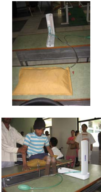
Fig. 4: Pillow manometer for push up clearance_:
