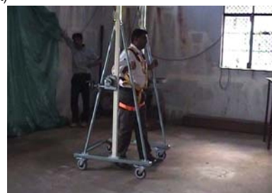
Fig. 2: Newly designed manual unweighing harness system for gait training(musgt)
