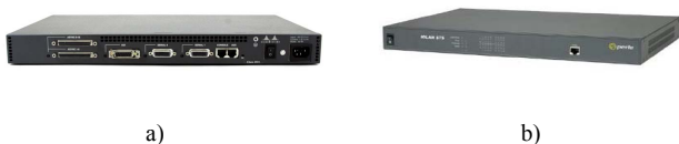
Fig. 6. Both middleware console servers used in the laboratory – a Cisco 2511 Access server (a) and a Perle STS 16 Iolan console server (b)
