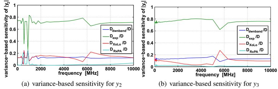
**Fig. 3** Global sensitivity analysis performed for an investigated floorplan model under input variations of 0.2 for every parameter.
