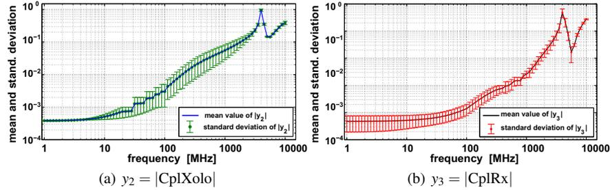
**Fig. 2** Mean and standard deviation values of the cross-domain transfer functions calculated for an investigated floorplan model under input variations of 0.2 for every parameter.
