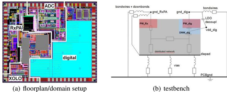
**Fig. 1** Chip architecture with domains indicated [3] (a) floorplan model for isolation and grounding strategies [5] (b) for a RFIC isolation problem.
