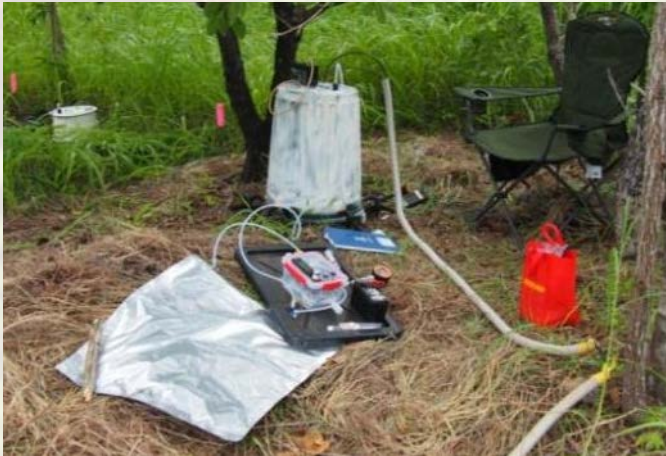
Injection of DFM into TM, while gas concentrations in the chamber headspace are monitored with the FGGA.
