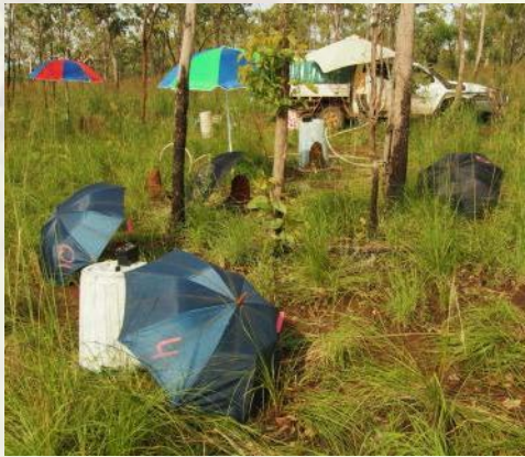
Field measurements of CH 4 and CO 2 emissions, and termite sampling in Northern Australian savannah in the wet season.
