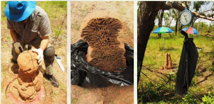
Selected mounds were cross-sectioned and the above-ground part was weighted to estimate the bulk density of the TM
