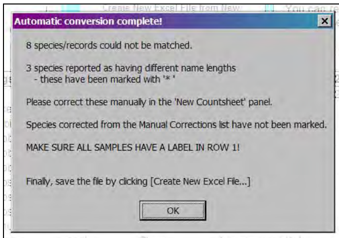
Figure 3.31. Screenshot: Message displayed on completion of the automatic phase of imported file conversion. All problems indicated here must be corrected manually in the File Converter before import can continue.
