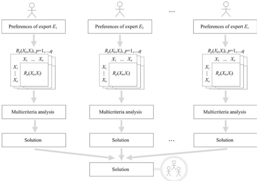
**Fig. 3** Aggregation of individual results (adapted from Pedrycz et al. (2010))
