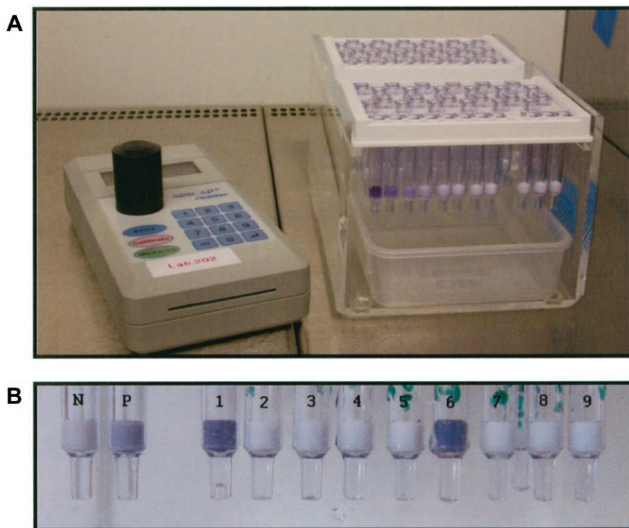
Figure 4. Immunofiltration assay. A , Photometer and rack with immunofiltration columns as used in the field. B , Results of a representative field test from Mbomo, Republic of the Congo. Patient serum samples are in columns 1–9. Samples 1 and 6 were positive for Zaire ebolavirus (ZEBOV) antigen (see also table 1, patients 1 and 2); all other serum samples were negative for ZEBOV antigen. The visual results were confirmed by photometric analysis. N, negative control serum sample; P, ZEBOV Mayinga as a positive control.
