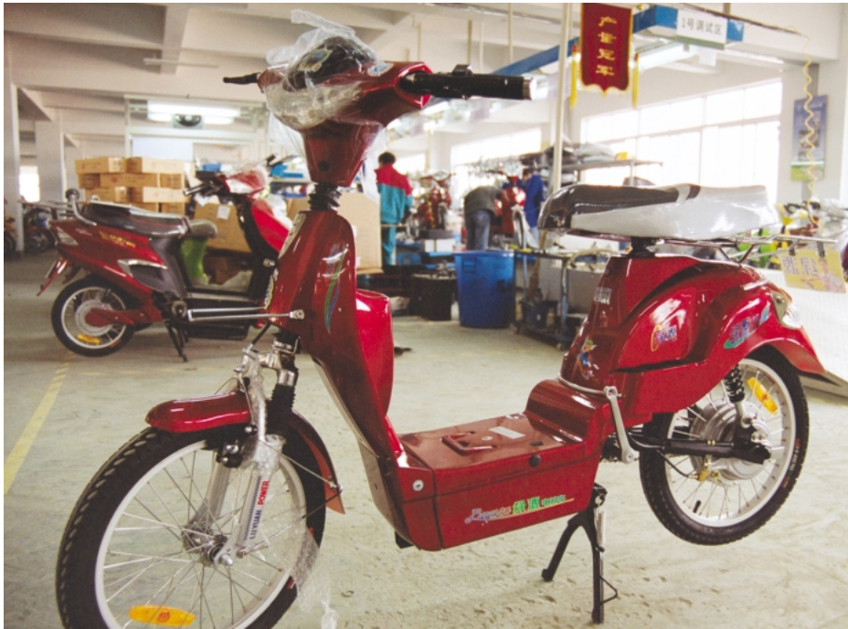
THE BASIC BIKE: The electric motor is in the rear wheel hub, and the removable battery is in the platform between the wheels. The electronic controller is between the handles.
