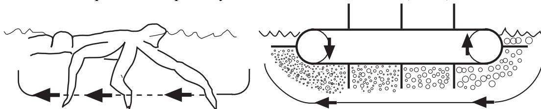
Figure 4: Early view on the mechanics of propulsion: The hand is used as an oar. The hand is pulled straight back, creating a high pressure zone on the palm, and a low pressure zone on the back of the hand. The resulting propulsive drag force would propel swimmers forward corresponding to the caterpillar paddle-wheel (right). However, in reality this form of propulsion is rather ineffective, because turbulence from one blade affects the ability of the following blade to create drag. Also, a relative small mass is given a rather large velocity change, leading to large losses of kinetic energy to the water .
