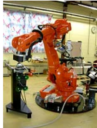
Fig. 2. Picture of one of the mobile fixtures and one robot on a platform
