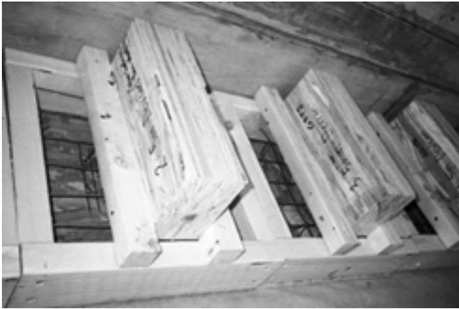
Figure 5. — Shear specimen formwork.
