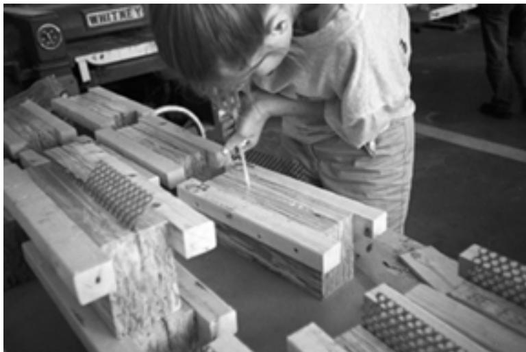
Figure 4.— Shear connectors being glued into rout in PSL member for shear specimens.
