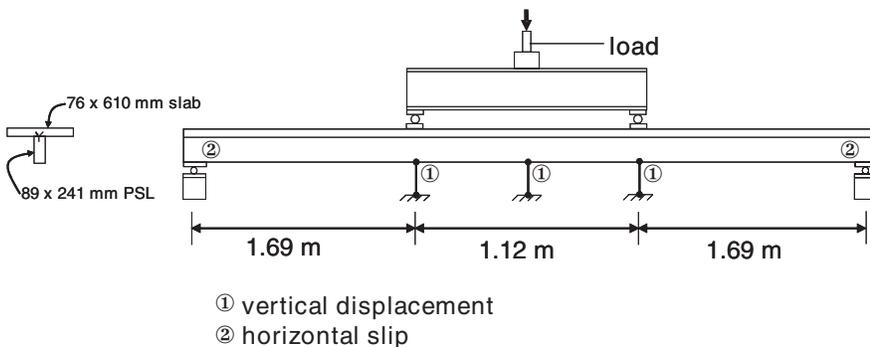
Figure 11. — Bending test set-up.
