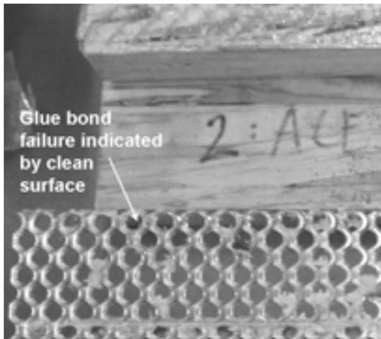
Figure 10. — Gluebond failure at steel surface.
