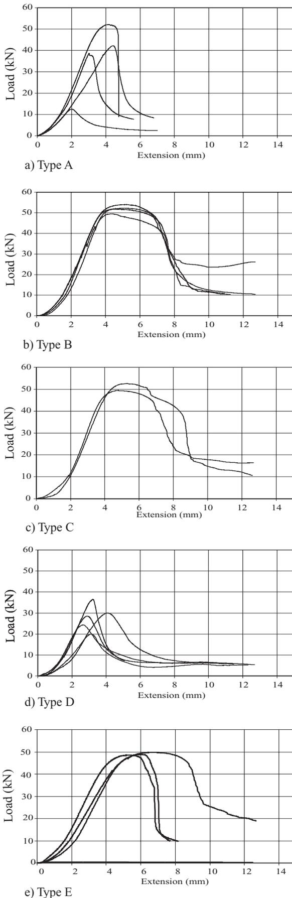
Figure 8. — Load vs. crosshead extension for shear tests.
