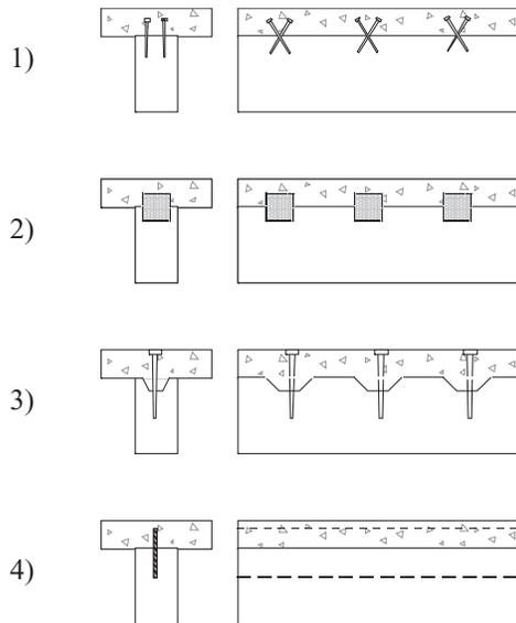
Figure 3.— Shear connector groups: 1) dowel; 2) tubular or metal plate; 3) shear key with anchor; and 4) (dis)continuous glued-in wood plate.
