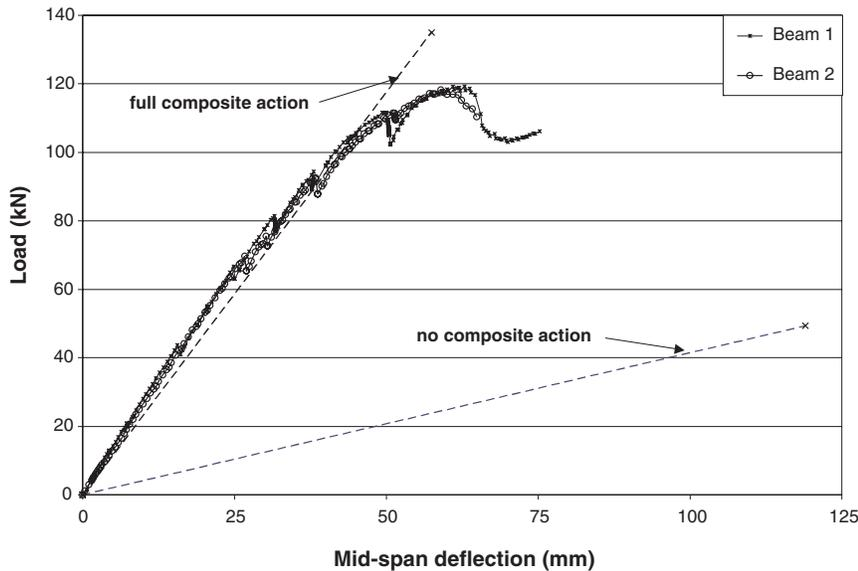
Figure 12. — Load versus mid-span displacement of composite beam specimens.
