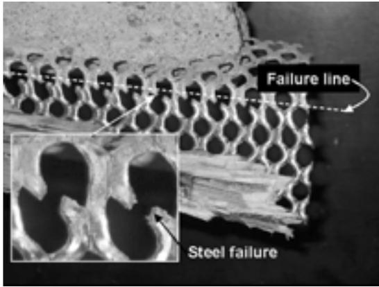
Figure 9. — Steel shear failure.
