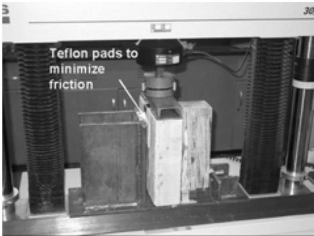
Figure 6. — Shear test set-up.
