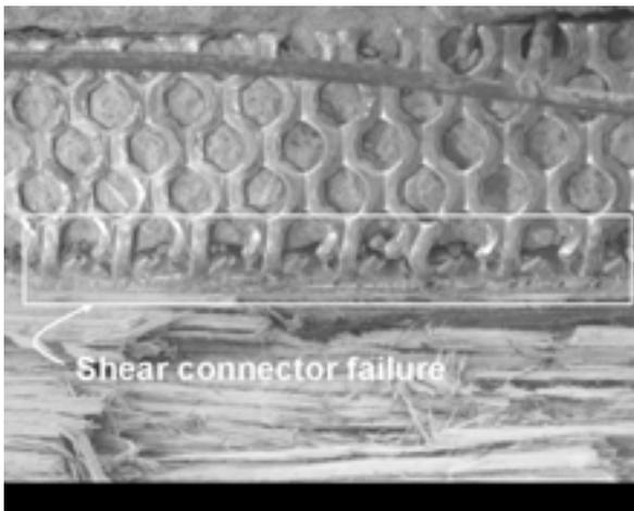
Figure 13. — Shear failure in steel mesh connector in composite beam specimen.
