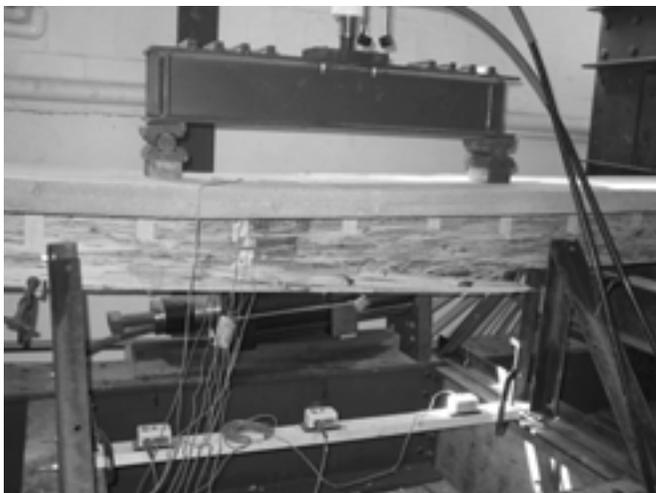
Figure 14. — Ultimate bending failure of wood-concrete composite beam.
