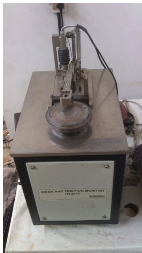
Figure 1. Pin on disc setup
