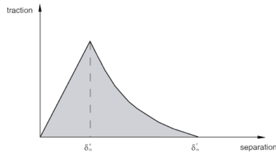
Fig. 5. schematic view of mortar degradation function
