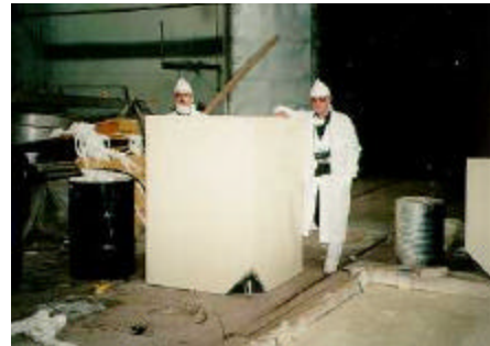
Figure 4. Solid radwaste container after spray coating with Polibrid 705.
