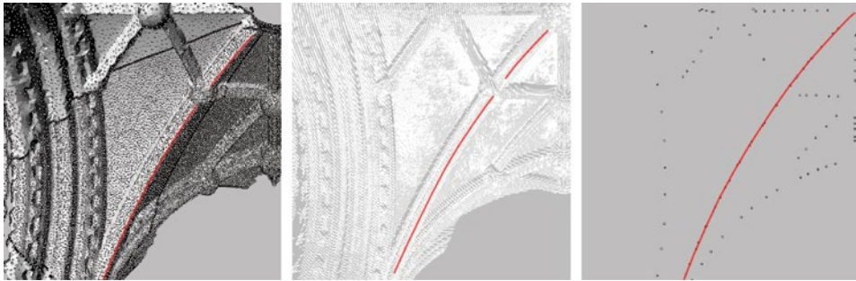
Fig.02. Three tracing methods used for the investigation. Mesh model (left), point cloud model (centre), and total station (right).
