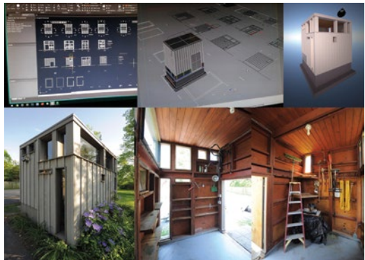
Fig. 03. Relatively small full-scale architectural models are derived in complex 2D and 3D digital drawings using Autocad and Rhino. Rhino, Revit and Maxwell are used to learn all the necessary drawing, modeling and rendering conventions.
