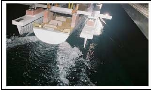
Figure 5: Center Hull @ 11.5 m Draft. Side Hulls in Aft Longitudinal & Inboard Transverse Location @ 7.5 m Draft - 35 Kns
