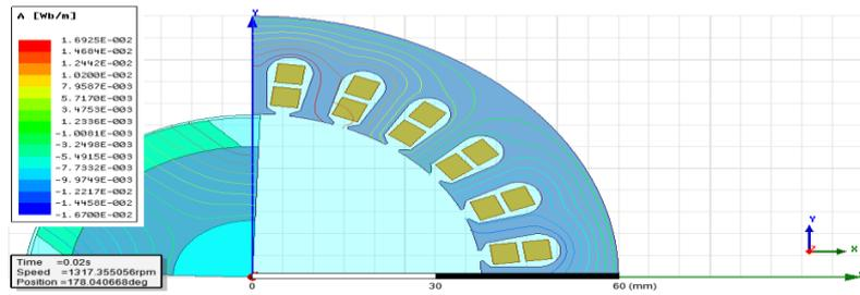
**Figure 12: Magnetic Flux Lines of Pole Type 2**
