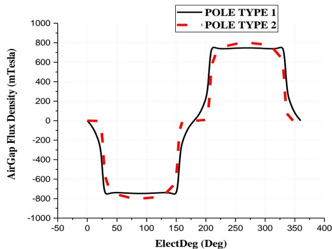
**Figure 7: Air gap Flux Density and Electric Degrees**
