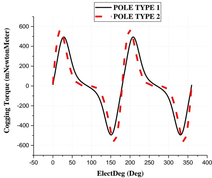
**Figure 8: Cogging Torque and Electric Degrees**
