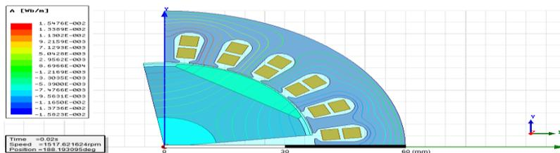
**Figure 10: Magnetic Flux Lines of Pole Type 1**
