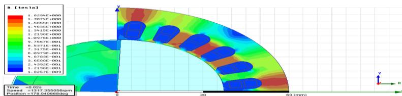
**Figure 11: Magnetic Flux Density of Pole Type 2**
