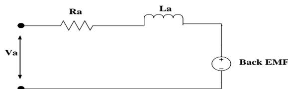
Figure 3: Single Phase Equivalent Circuit of Brushless PMDC Motor
