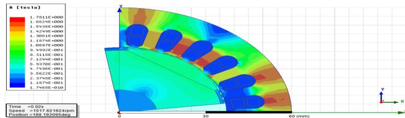
**Figure 9: Magnetic Flux Density of Pole Type 1**
