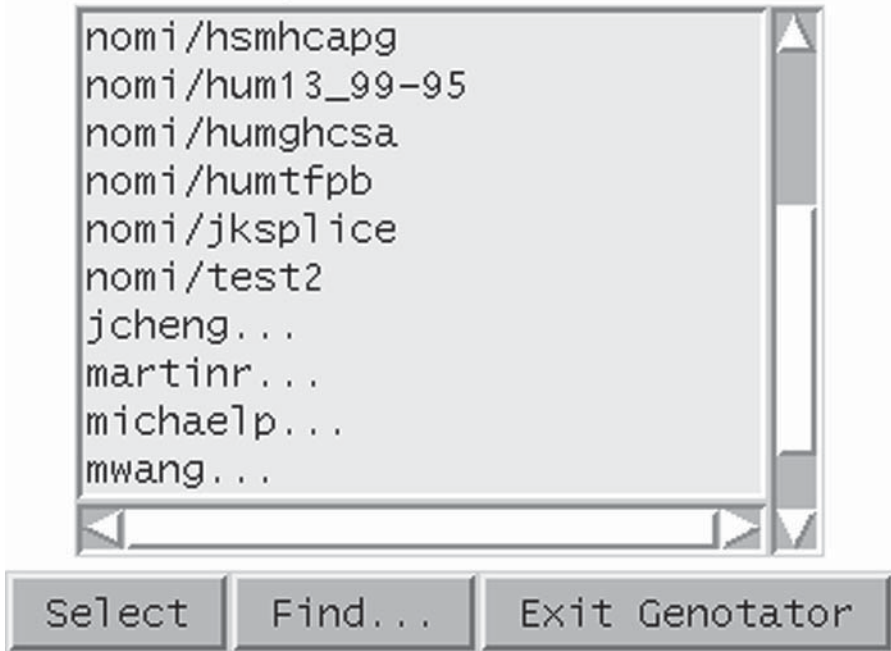
Fig. 2. If the Genotator browser is invoked with no arguments, it brings up a list of annotated sequences. Directories that are not owned by the current user are collapsed and indicated with "...".
