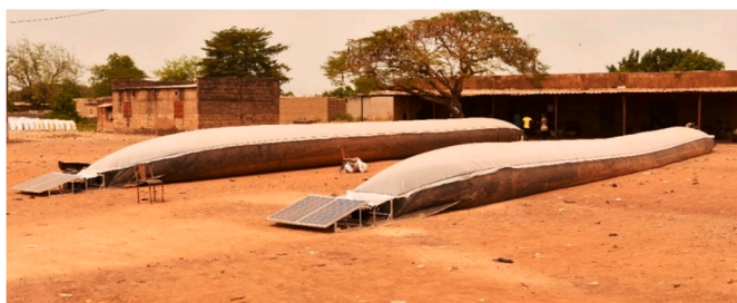
Fig. 7. Application of inflatable solar dryers to dry paddy rice in Burkina Faso.
